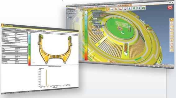
Advanced analysis such as wall thickness checks or the detection of small holes and other details can be used to identify critical areas for specific processes. Furthermore, the internal backlash check and undercut analysis allows to identification of problem areas or models with particularly good 3D printing potential. In the interplay of all functions and the intelligent scripting language, 3D models can be pre-sorted quickly and easily.
