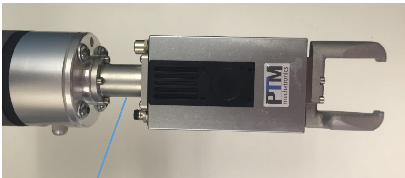
The active magnetic break is integrated in the robot flange
