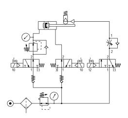
$For a correct use of the rod lock \verb|Mod.RLC| a pneumatic connection| is recommended (as shown in the examples).$
