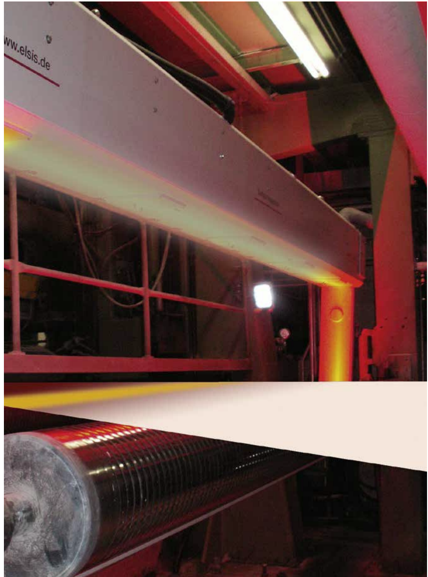
A protection rating up to IP 54 also makes it possible to integrate inspection in harsh environments
