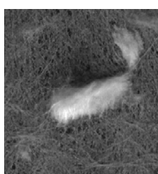
Defect example: tangle
