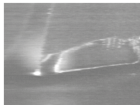
Defect example: missing coating
