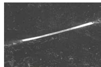
Defect example: crease
