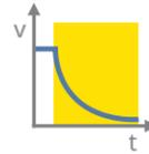
STO safely interrupts the power supply to the motor in the servo drive. The motor becomes torque-free.
