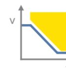
The drive is brought to a standstill by controlled braking and subsequently remains in controlled standstill. The control functions of the drive are maintained.
