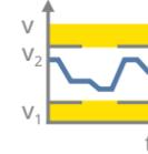
Monitors that the drive observes a defined speed range. In the event of an error, SS1 is triggered.
