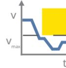
Monitors that the drive observes a defined speed limit. In the event of an error, SS1 is triggered.
