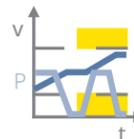
Monitors the absolute position of the drive. If the limit value is reached or the brake torque is too low to keep the drive within the limit value, SS1 is triggered.
