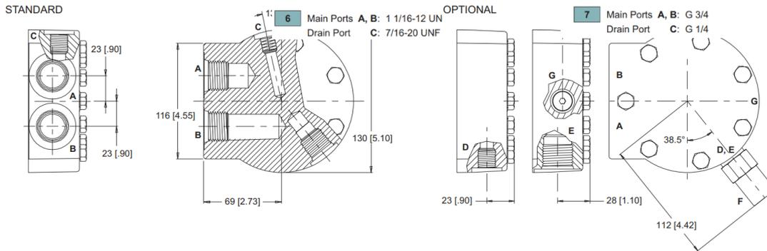
D: Internal Drain E: 10 Series/2-Way Valve Cavity 7/8-14 UNF F: Valve Cartridge Installed G: Internal Drain Placement With Valve Cavity
