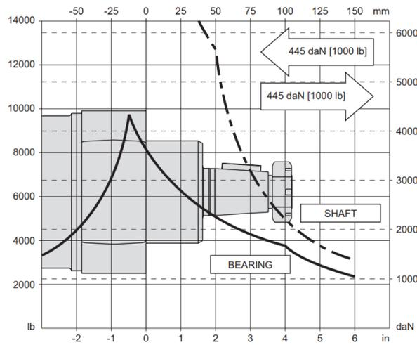
Figure 31 DR 630 Allowable Shaft Load/ Bearing Curve
