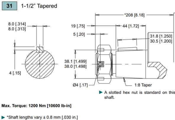
Figure 26 1-1/2 Tapered Shaft
