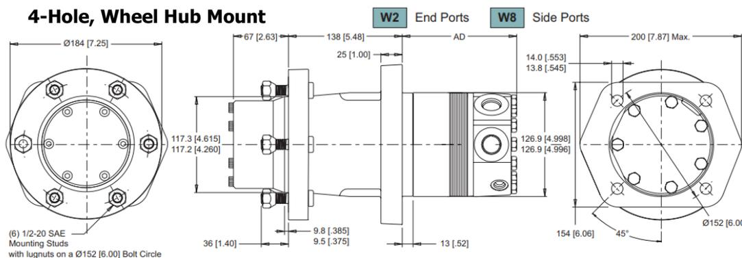
Figure 45 DT 740 4-hole (Wheel Hub Mount)
