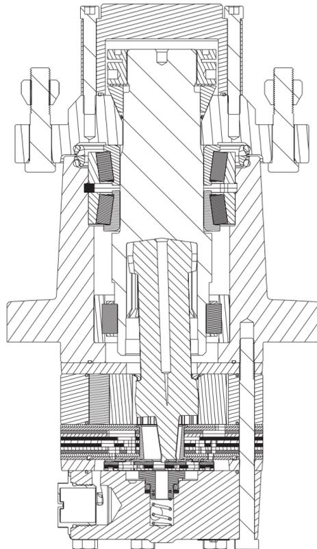
Figure 38 DT 740 Hydraulic Motor with Wheel Hub
