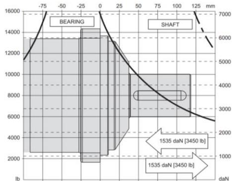
Figure 52 160 mm PILOT Wheel Mounts Allowable shaft load/ bearing curve
