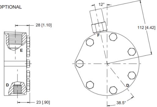
D: Internal Drain E: 10 Series/2-Way Valve Cavity 7/8-14 UNF F: Valve Cartridge Installed
