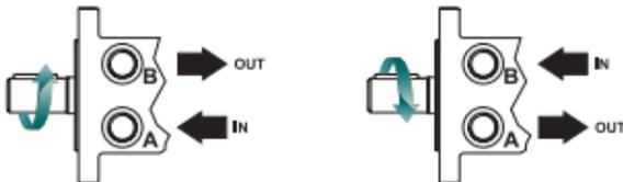
▶ The 630 series is bi-directional. Reversing the inlet hose will reverse shaft rotation.
