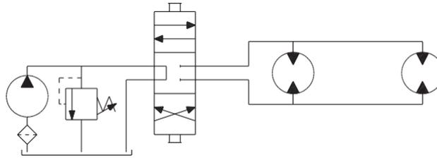
Figure 3 Parallel connection
