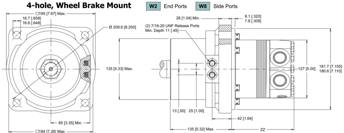
Figure 24 DR 610 Series, 4-hole Wheel Brake Mount
