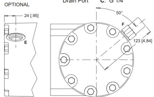
E: 10 Series/2-Way Valve Cavity 7/8-14 UNF F: Valve Cartridge Installed
