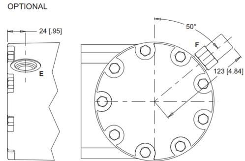
E: 10 Series/2-Way Valve Cavity 7/8-14 UNF F: Valve Cartridge Installed
