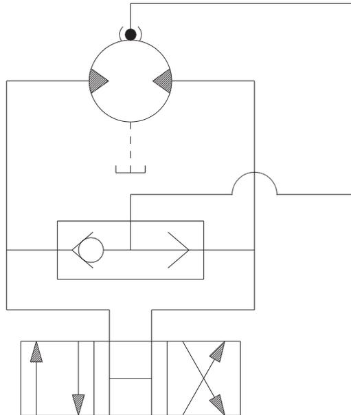
Figure 1 Typical Motor/ Brake schematic
