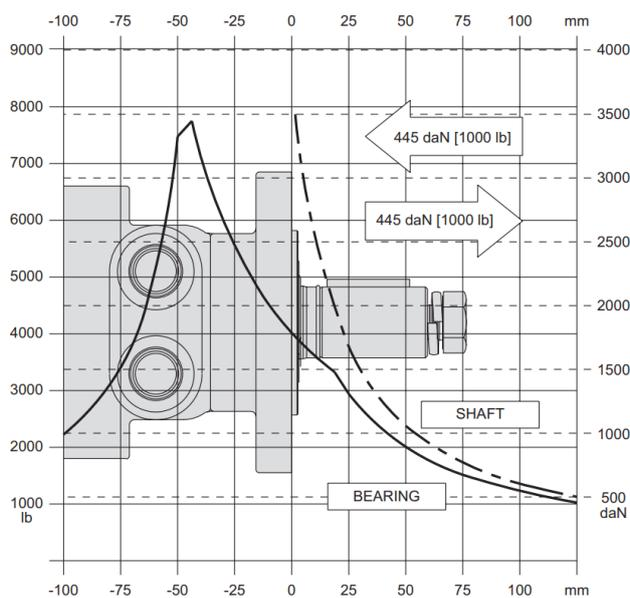
Figure 5 Bearing and shaft loading
