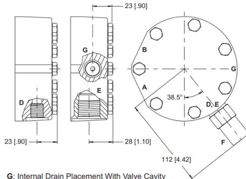
D: Internal Drain E: 10 Series/2-Way Valve Cavity 7/8-14 UNF F: Valve Cartridge Installed G: Internal Drain Placement With Valve Cavity
