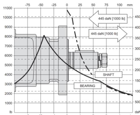
Figure 28 DR 620 Allowable Shaft Load/ Bearing Curve
