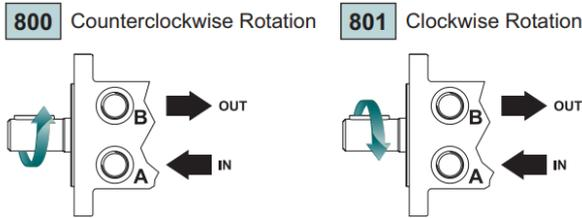
► The 800 & 801 series are bi-directional. Reversing the inlet hose will reverse shaft rotation.
