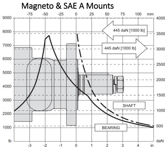
Figure 22 Magneto & SAE A Mounts Allowable Shaft Load / Bearing Curve
