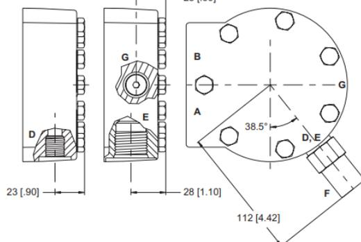
D: Internal Drain E: 10 Series/2-Way Valve Cavity 7/8-14 UNF F: Valve Cartridge Installed G: Internal Drain Placement With Valve Cavity
