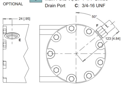
E: 10 Series/2-Way Valve Cavity 7/8-14 UNF F: Valve Cartridge Installed
