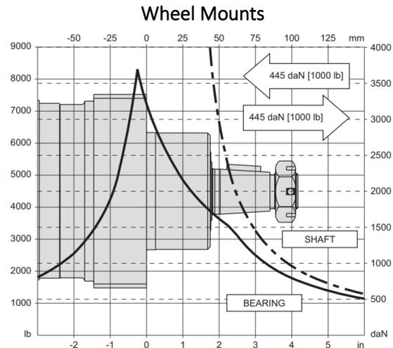
Figure 23 Wheel Mounts Allowable Shaft Load / Bearing Curve
