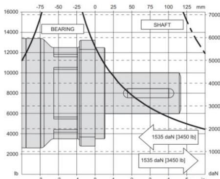
Figure 51 SAE C Mounts Allowable shaft load/ bearing curve
