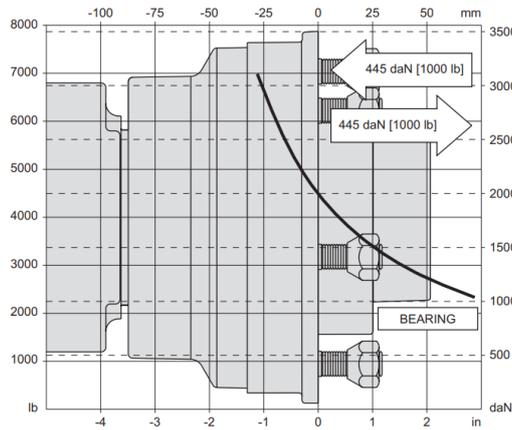
Figure 36 Wheel Hub Mounts Allowable Shaft Load / Bearing Curve
