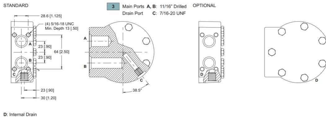
Figure 17 DR Porting (manifold aligned)
