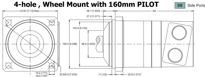
Figure 49 D9 Wheel Mount with 160 mm PILOT
