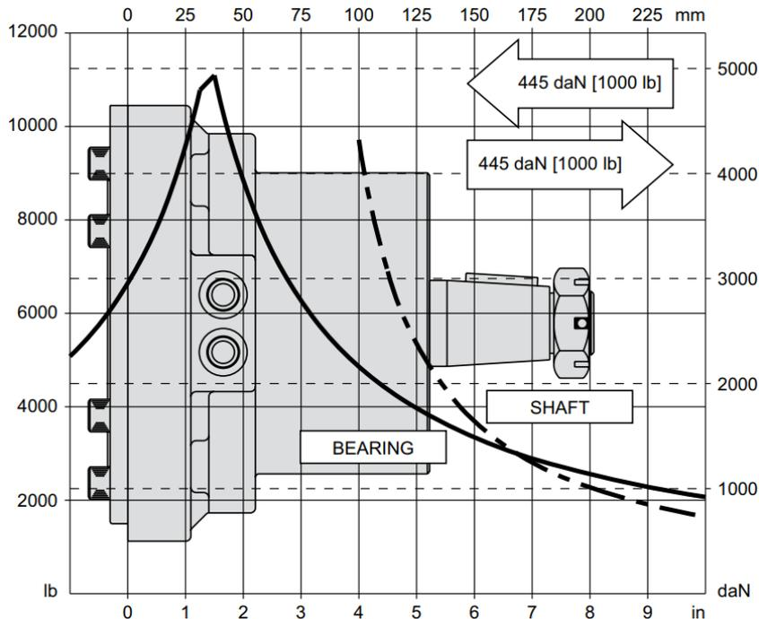
Figure 25 Wheel Brake Mount Allowable Shaft Load/Bearing Curve
