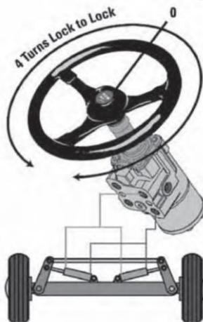
Figure 27 Traditional Metered Steering
