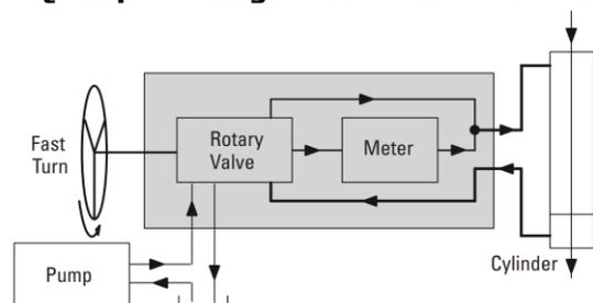
Figure 18 Q-Amp Steering Control Unit – Fast Turn
