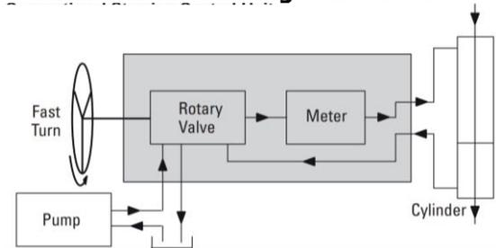
Figure 17 Conventional Steering Control Unit
