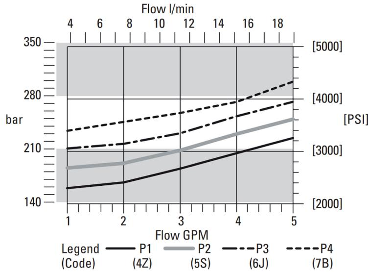
Figure 42 Cylinder Relief Valve Pressure
