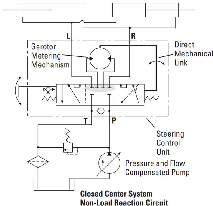
Figure 9 Closed Center System (Non-Load Reaction Circuit)
