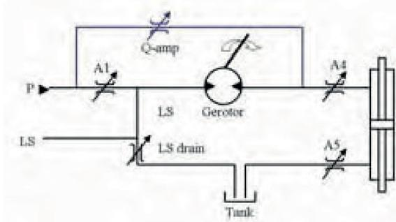
Figure 23 Flow Amplification without Cylinder Damping
