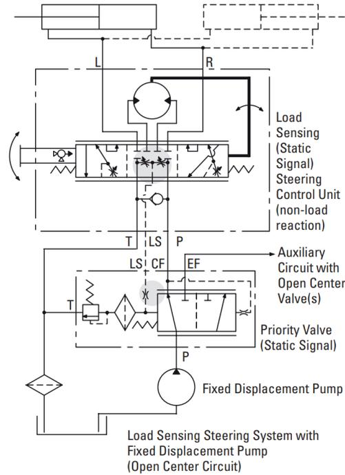
Figure 8 Static Signal
