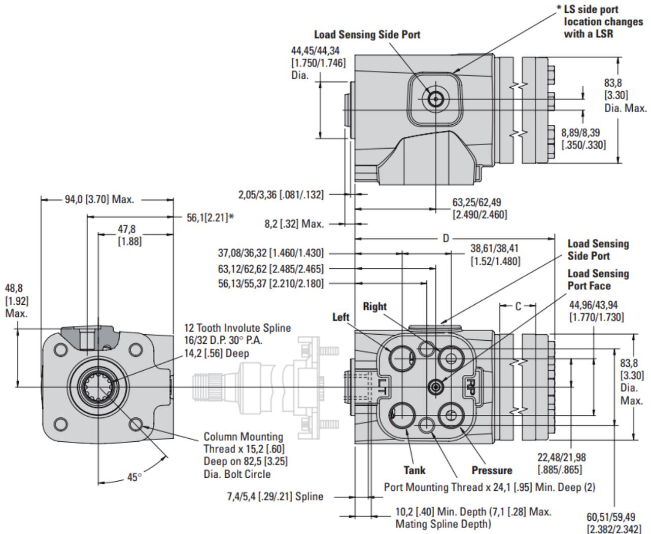
Figure 31 Installation Drawing
