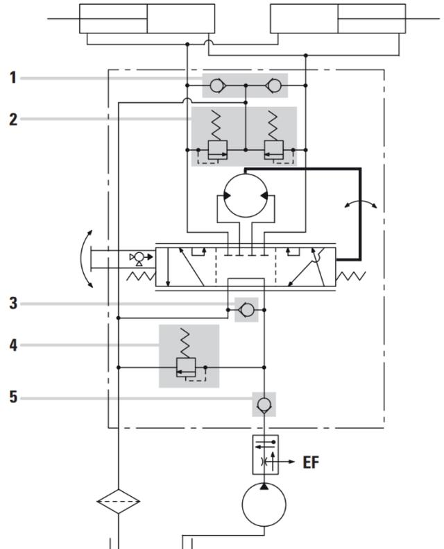
Figure 11 Steering Units with Integral Valves
