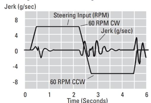
Figure 22 Wide Angle Steering on a 25 Ton Loader
