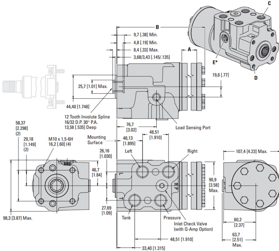
Figure 39 20 Series Installation Drawing
