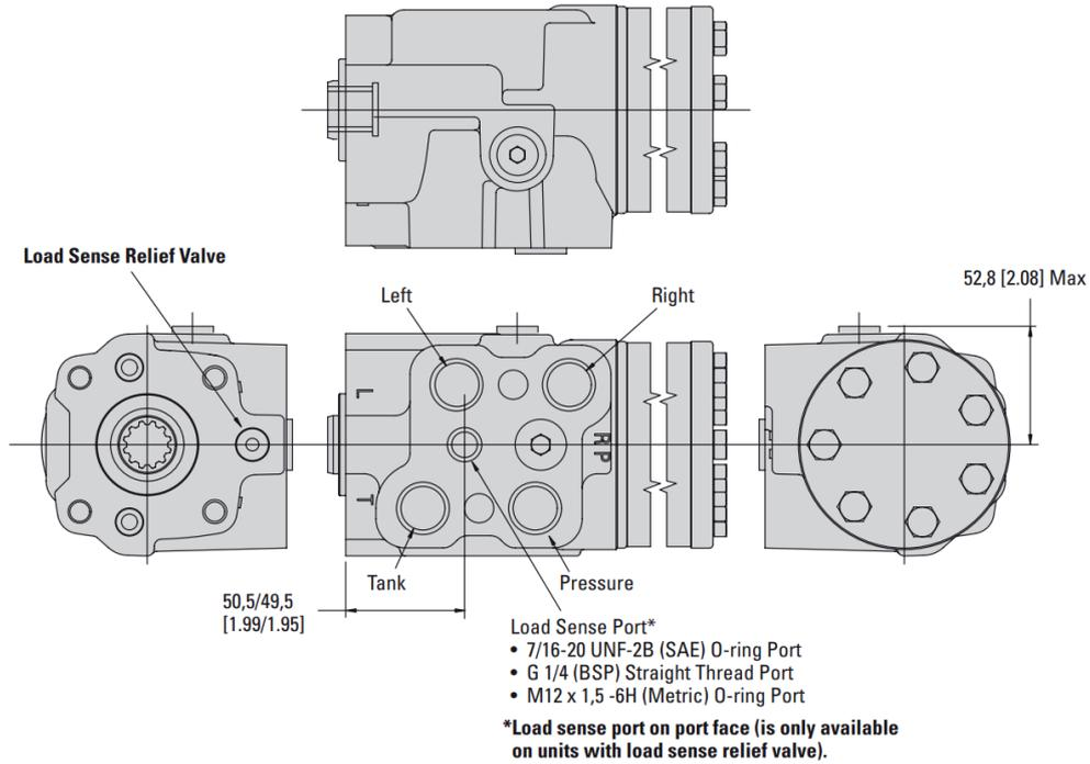
Figure 40 Installation Drawing (Load Sense Relief Option)
