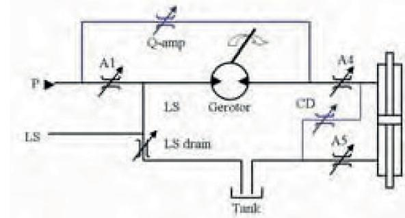
Figure 24 Flow Amplification with Cylinder Damping
