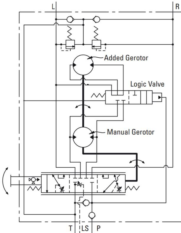
Figure 14 Dual Displacement
