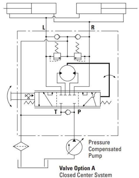
Figure 3 Valve Option A (Closed Center System)
