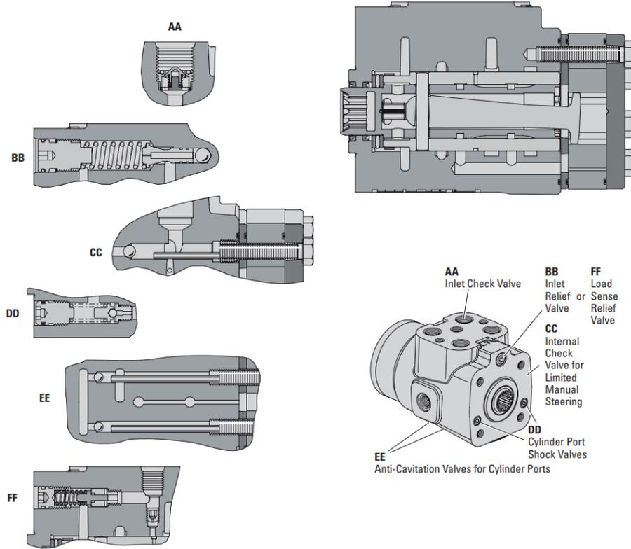
Figure 32 Sectional Drawing and Integral Valves
