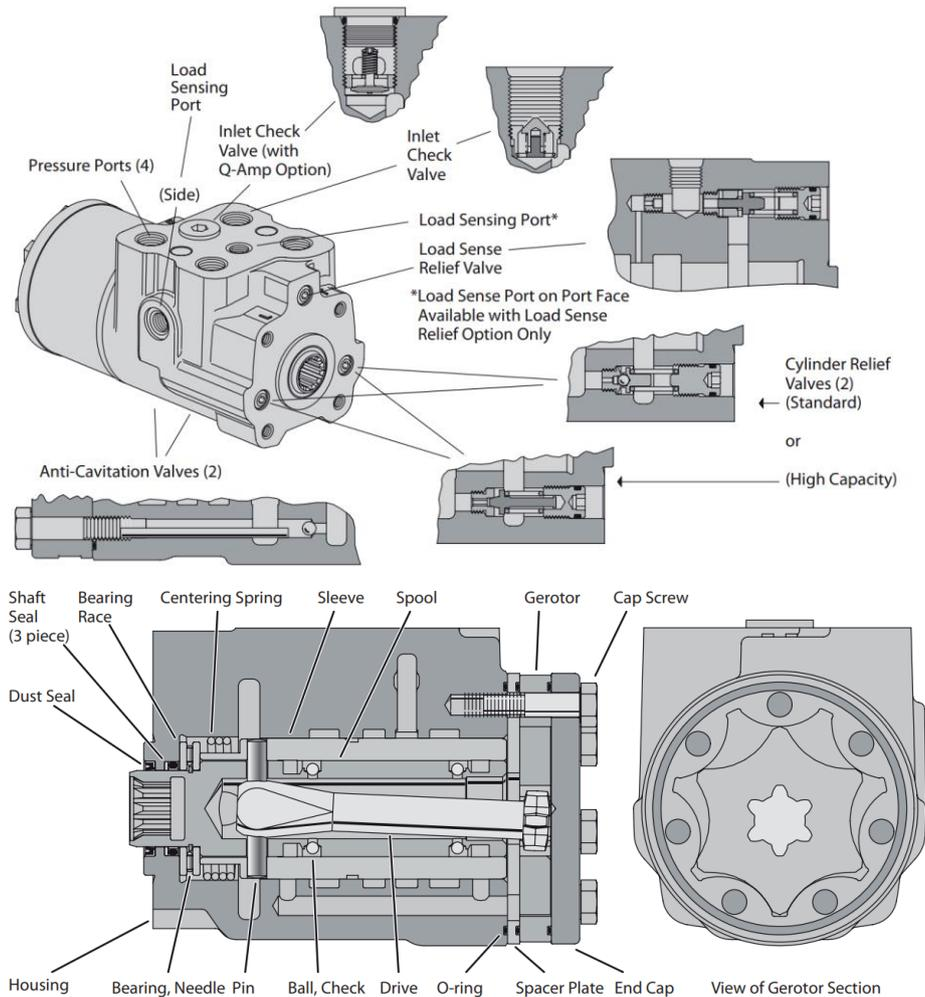
Figure 41 Sectional Drawing and Integral Valves
