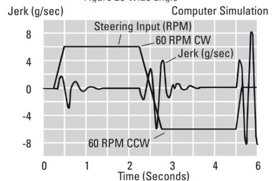
Figure 21 Standard Steering on a 25 Ton Loader
