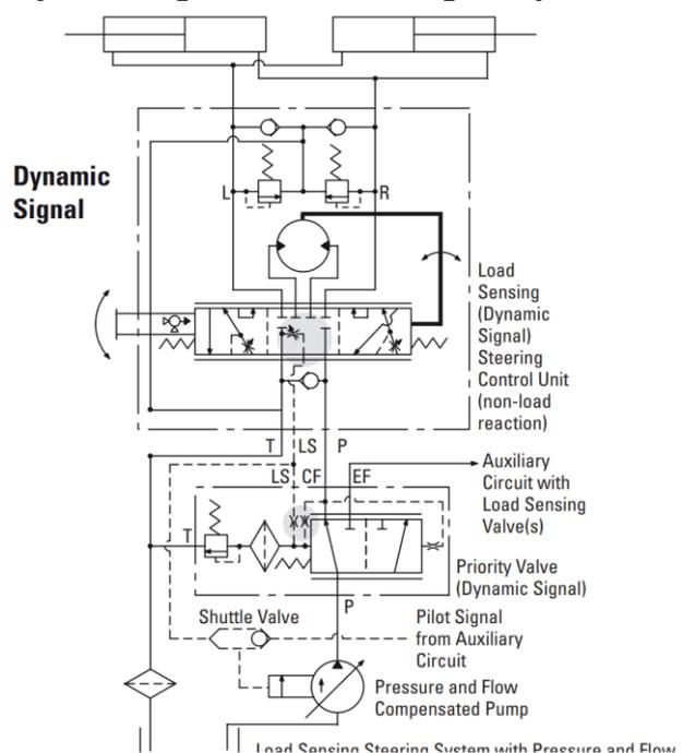
Figure 7 Dynamic Signal—Load Sensing Pump
