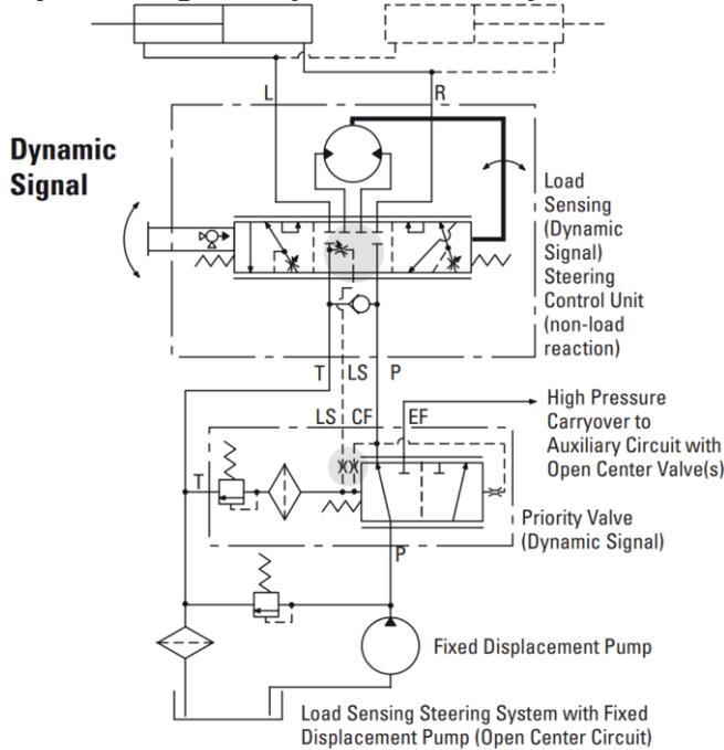
Figure 6 Dynamic Signal—Open Center Pump
