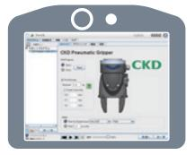
The total mass (Payload) and the position of the center of gravity can be set for tools necessary for robot operation when configuring gripper settings.
