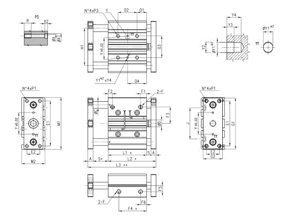
In case of use of lateral ports, unscrew the related threaded caps, screw them in the front ports and tighten them up to the cylinder surface (not tighter) having care to use a proper sealer.
