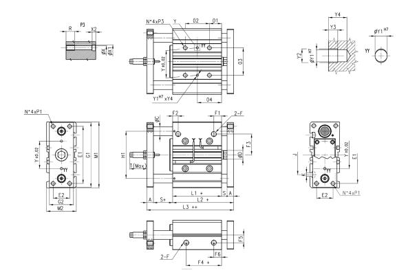
In case of use of lateral ports, unscrew the related threaded caps, screw them in the front ports and tighten them up to the cylinder surface (not tighter) having care to use a proper sealer.
