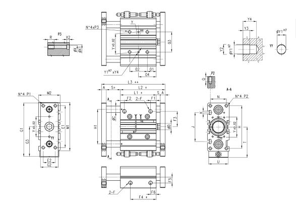
In case of use of lateral ports, unscrew the related threaded caps, screw them in the front ports and tighten them up to the cylinder surface (not tighter) having care to use a proper sealer.
