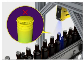
Ensure bottles are properly sealed by checking the height and angle of the bottle cap.
