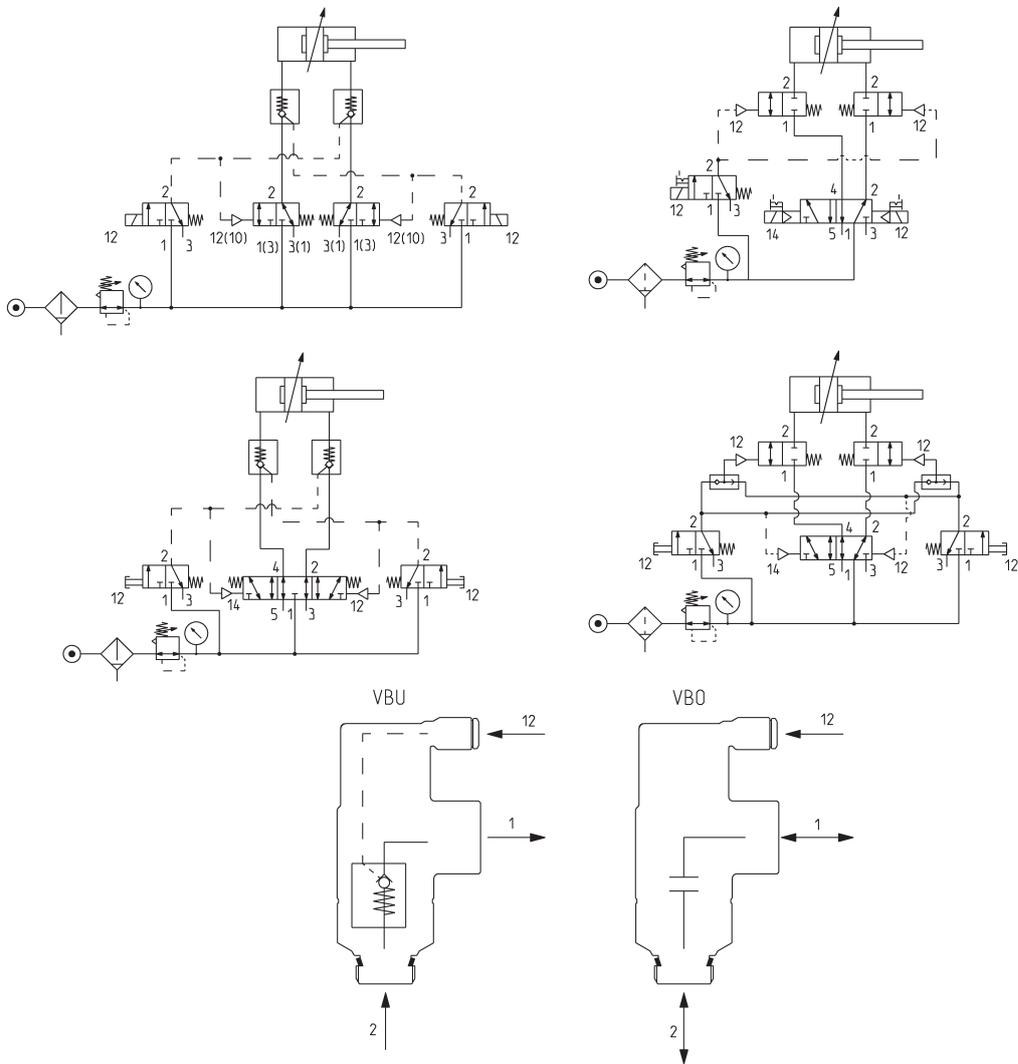
STOPVENTILE, RÜCKSCHLAGVENTILE SERIE VBO UND VBU
