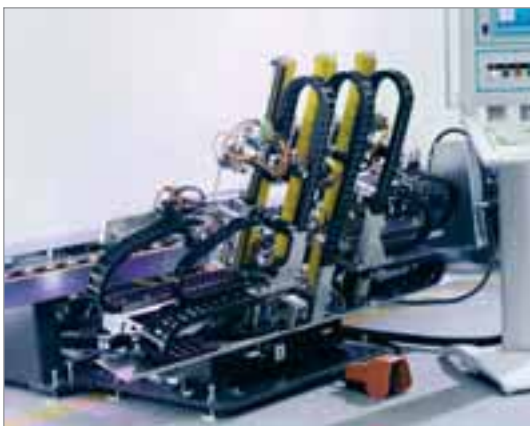
UNIFLEX Series cable carriers on an automatic stove setting station Photographs: Lenhard Maschinenbau GmbH
