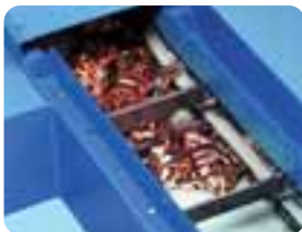
Scraper conveyors – for disposal of small materials
