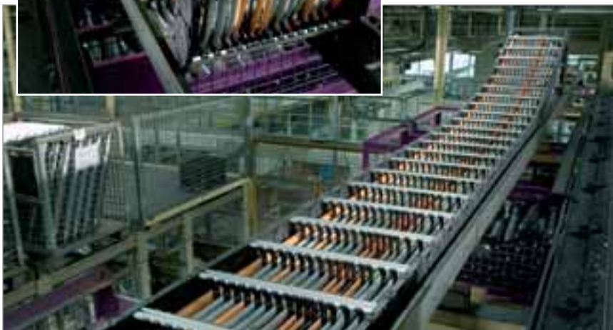
M Series cable and hose carriers on a highrise rack
