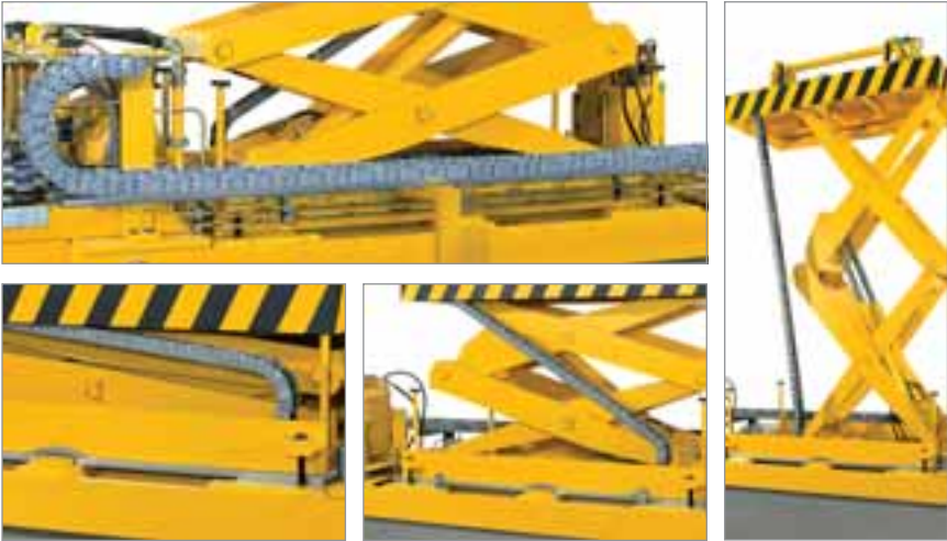
Steel cable carriers on a scissored coil lift Photographs: SÜDO GmbH
