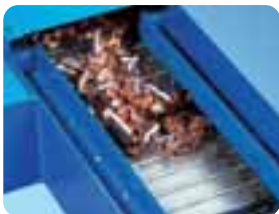
Hinged belt conveyors – proven for a wide range of disposal tasks
