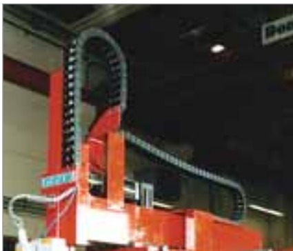
MONO Series cable carrier systems, type 0450 Installation variants: horizontal "unsupported" – and vertical "standing" Photograph: Reis Robotics
