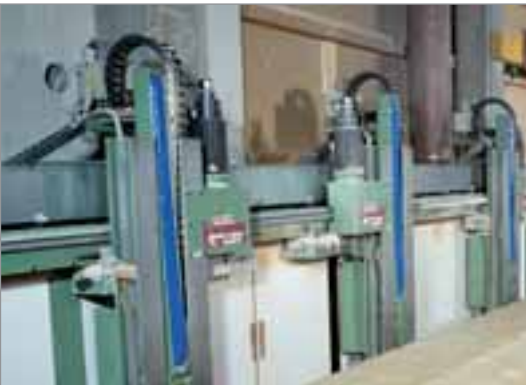
MONO Series cable and hose carriers on a wood processing machine
