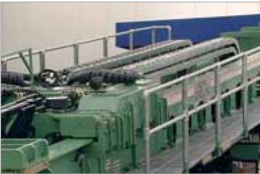
Steel cable carriers on a drilling system Photograph: Prime Drilling GmbH
