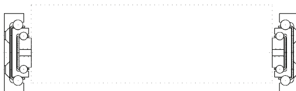
Standard application: Drawer extension telescopic rails vertical.
