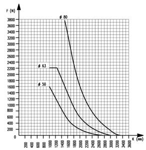
This chart has been made according to a max. distance of 0.5 mm Load (N).
