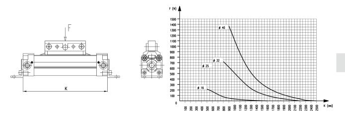
This chart has been made according to a max. distance of 0.5 mm Load (N). Once the load and the cylinder diameter have been fixed, the chart gives the K values beyond which it is necessary to put an intermediate feet Mod. BH-50.
