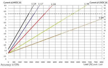
Recommended max. current: 12VDC = 16A and 24VDC = 8A
