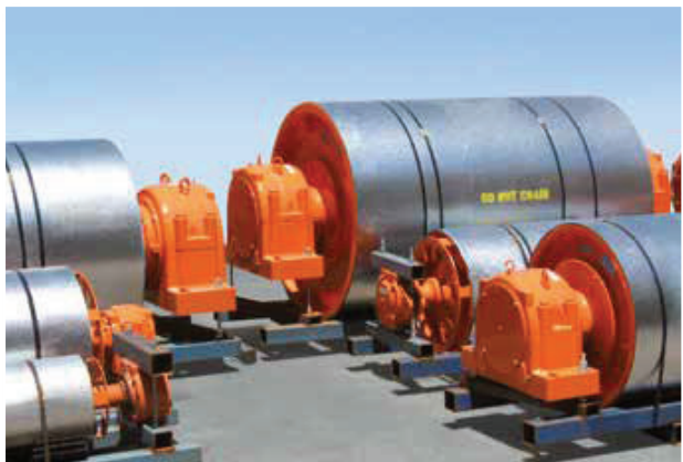
Ready-for-shipping belt drum with Locking Assemblies
