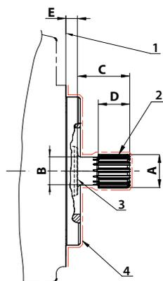
1. Surface of mounting flange 101 – 2 per ISO 3019-1 (SAE B); to be paint free
