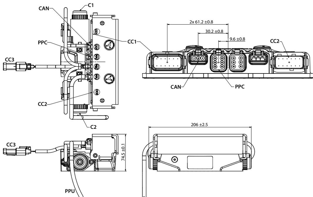
PPU wire harness is factory installed to speed sensor.
