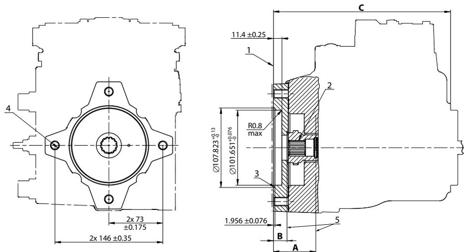
1. Auxiliary mounting pad for mating flange 101-2 per ISO 3019-1 (SAE B); Paint free
