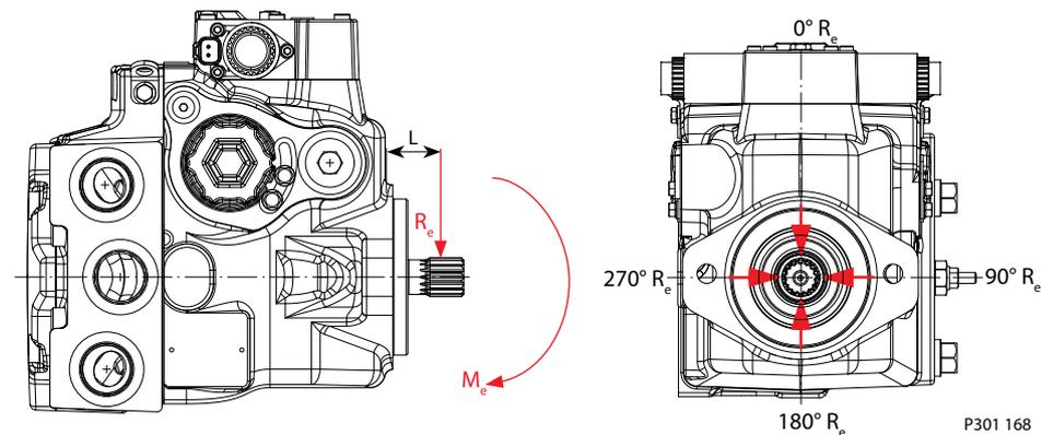
The maximum allowable radial shaft load ( $R_e$ ) is based on the maximum external moment ( $M_e$ ) and the distance ( $L$ ) from the mounting flange to the load. It may be determined using the following formula:
