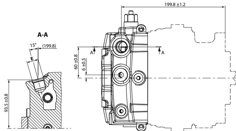
**E** Charge filtration ports per ISO 11926-1:  $\frac{7}{8}$ -14 from filter
