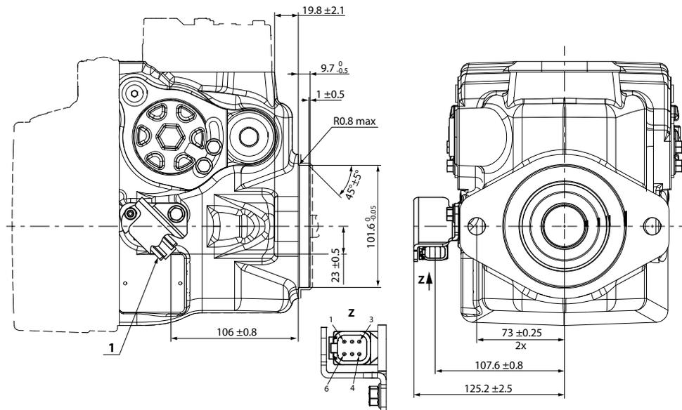
1. Speed sensor connector DEUTSCH DTM04-6P, paint free
