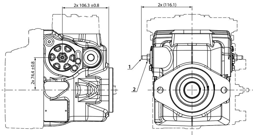
1. Displacement limiter screw (2x)
