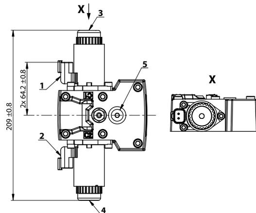
1. Control solenoid connector **C1** DEUTSCH DT04-2P, paint free
