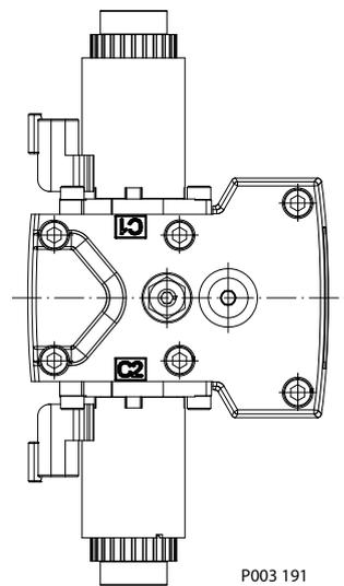
*EDC schematic, feedback from swash plate*
