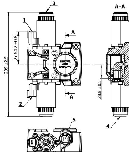
1. Control solenoid connector **C1** DEUTSCH DT04-2P, paint free
