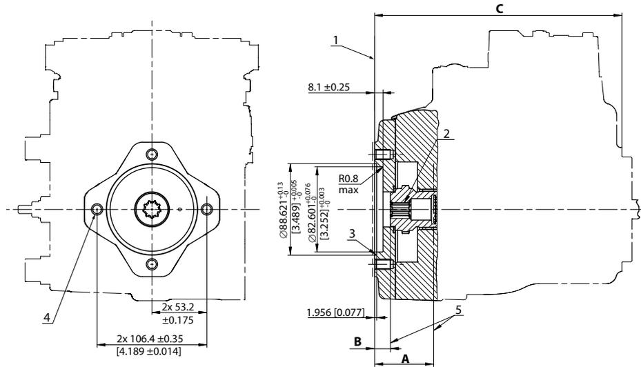
1. Auxiliary mounting pad for mating flange 82-2 per ISO 3019-1 (SAE A); Paint free
