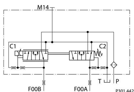
The pump should be configured with 0.8 mm control orifices to provide slowest response and maximize system stability. Additionally, pressure limiter (PL) valves are used to limit maximum fan trim speed in both (forward and reverse) directions.
