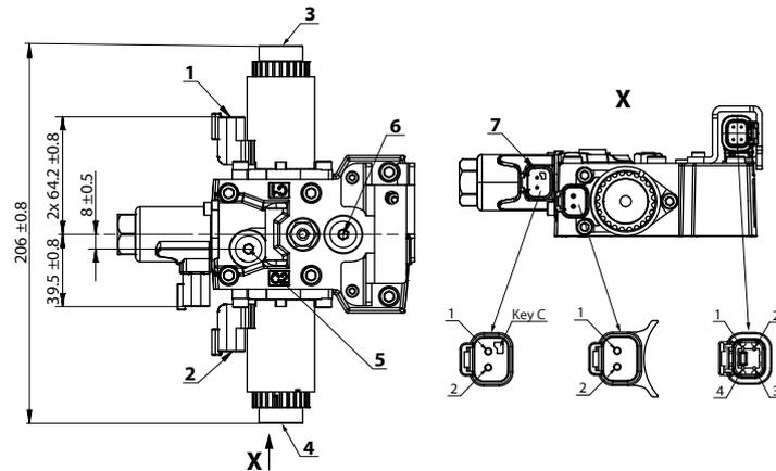
1. Control solenoid connector **C1** DEUTSCH DT04-2P, paint free
