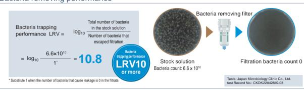
Verification data from test done based on JIS K 3835
