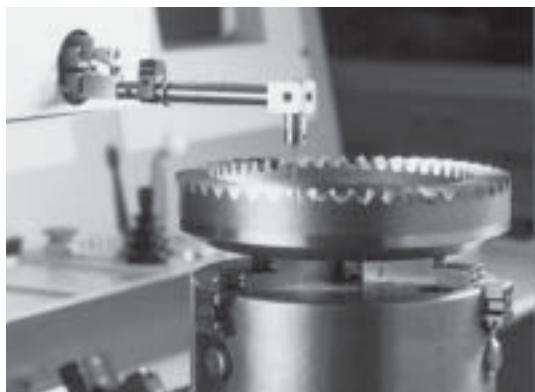
Computerized mapping of gear tooth profile
