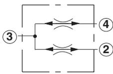
Note: Closed centre valves have spring centred internal spools that provide blocked flow paths when centred. Centring occurs when the Port 3 flow is also blocked. This internal blocking isolates Port 2 and 4 from cross flow.
