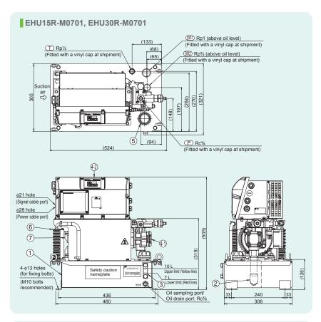
Do not place any obstacles to oil cooler air intake and exhaust within a distance of 100 mm from end faces of the unit. Install the unit at a location with good air flow so that heated air can be vented and take care about the temperature of the suction air: it must satisfy the stipulated condition for ambient temperature.
