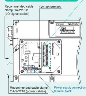
\* Main power supply connections: Connect a 3-phase AC power supply (200 V/50 Hz, 200 V/60 Hz, or 220 V/60 Hz) to the power supply terminals (L1, L2 and L3), and connect a ground cable to the ground terminal.
