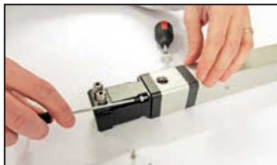
Tighten motor mounting screws
