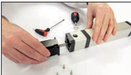
Insert motor shaft into coupling
