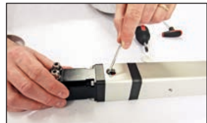
Tighten motor coupling screws and install sealing plug
