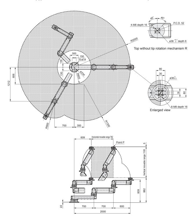
Shows dimensions with tip rotation mechanism R. Plane view shows movable view at the point P descending edge. Structurally, the movable range changes according to the point P rising height.
