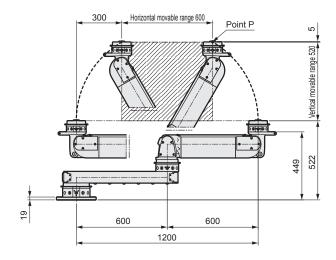
Shows dimensions with tip rotation mechanism R. Plane view shows movable view at the point P descending edge. Structurally, the movable range changes according to the point P rising height.
