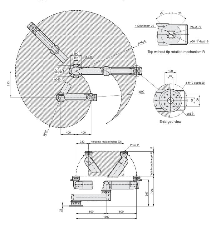
Shows dimensions with tip rotation mechanism R. Plane view shows movable view at the point P descending edge. Structurally, the movable range changes according to the point P rising height.
