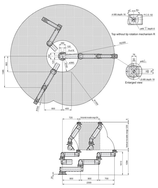
Shows dimensions with tip rotation mechanism R.
