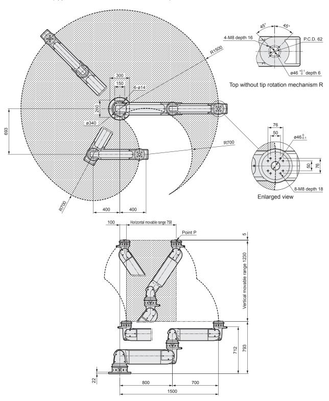
Shows dimensions with tip rotation mechanism R.
