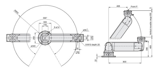
Shows dimensions with tip rotation mechanism R.
