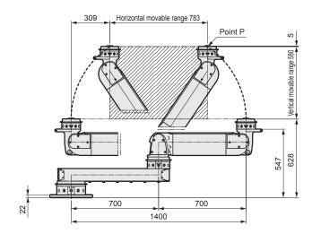
Shows dimensions with tip rotation mechanism R. Plane view shows movable view at the point P descending edge. Structurally, the movable range changes according to the point P rising height.
