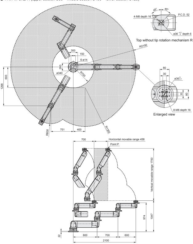
Shows dimensions with tip rotation mechanism R.
