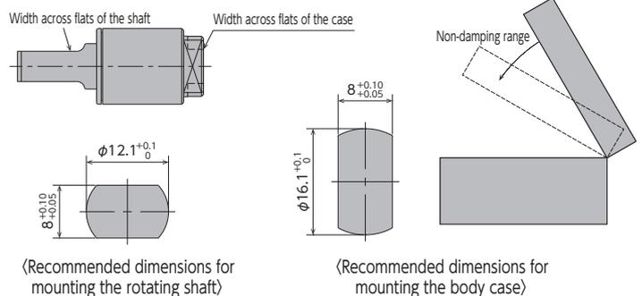
(Recommended dimensions for mounting the rotating shaft)
