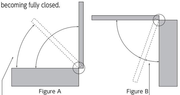
Stronger damper torque allows the lid to close gently until it is fully closed.
