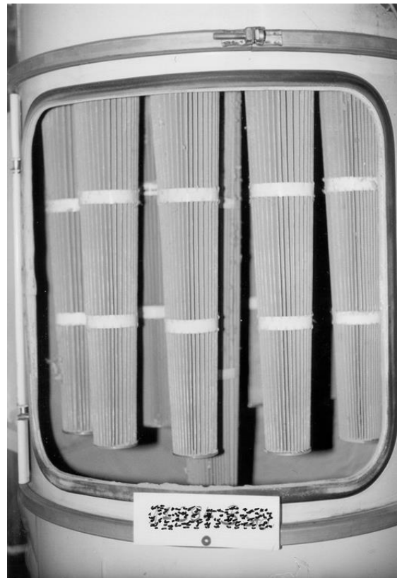
After changing to conical filter cartridges and 4,600 working hours.. Cartridges cleaned over the whole length.
