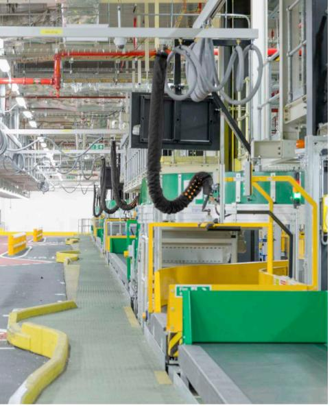
We recommend mounting your TAWI High frequency lifter in our own range of crane systems. The jib arm or bridge crane suspends the lift tube and is available in different lengths and capacities.
