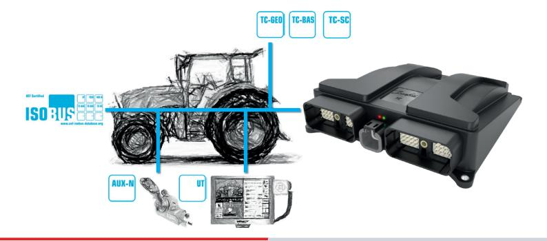
With the new XL104 controller series, you can integrate your attachment seamlessly into the ISO bus of tractor units. The powerful and flexible platform impresses with its high computing power, numerous interfaces and functional safety. Develop your application intuitively with the PLUS+1® GUIDE software environment - for the efficient machine management of tomorrow.
