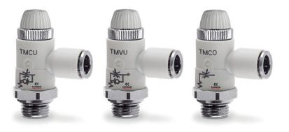
Series TMCU, TMVU, TMCO unidirectional and bidirectional flow controllers have been revised in order to decrease their dimensions and improve their flow rate characteristics. Their construction allows for easy assembly to cylinders and valves and allows the regulation adjustment to be precise and gradual.
