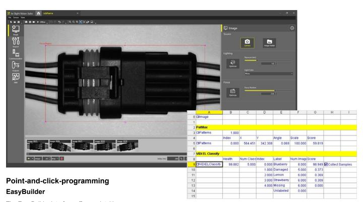
The EasyBuilder interface offers an intuitive, wizard-like experience that guides users step-by-step through setup of standard vision applications.
