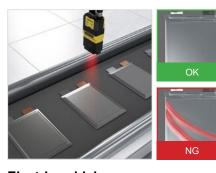
Electric vehicle Presence/absence detection: Find defects on EV battery pouches
