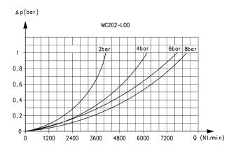
Flow diagram for model: MC202-L00
