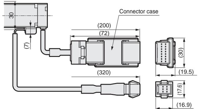
● **FLSH-20GH118NCN-F/S\*** (Stroke: 18mm, rubber cover: none, finger: basic, cable outlet type/direction: direct outlet)
