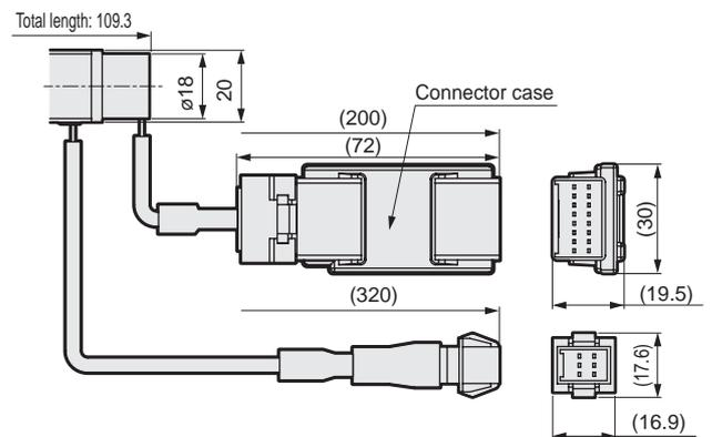
● FLSH-16GH112NCN-F/S\* (Stroke: 12mm, rubber cover: none, finger: basic, cable outlet type/direction: direct outlet)
