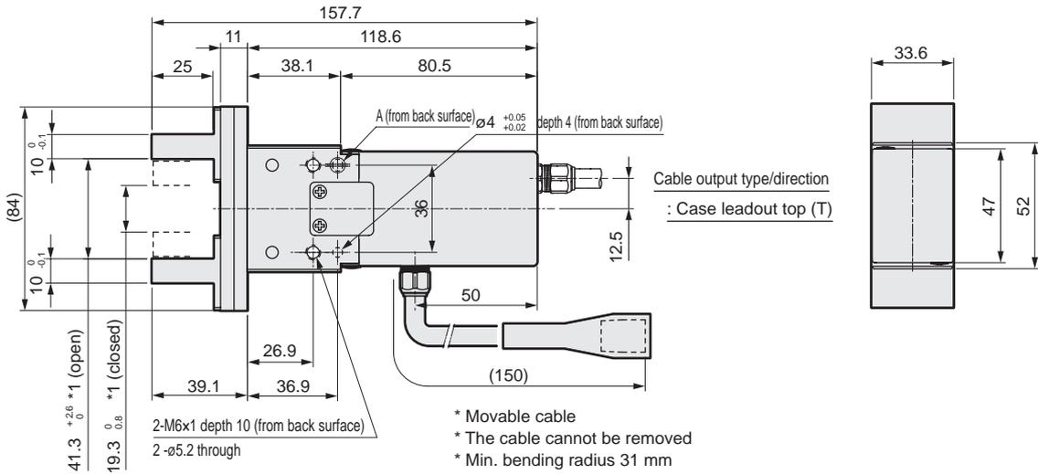
Cable output type/direction : Case leadout top (T)
