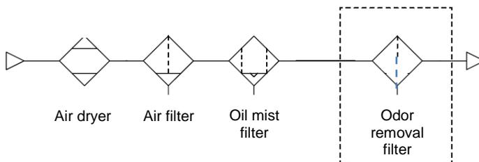
**Make sure that substances such as chlorine do not become mixed with the compressed air when using a water lubricated type compressor circuit.**
