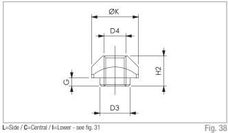
Steel nuts to be used in the slots of the body.
