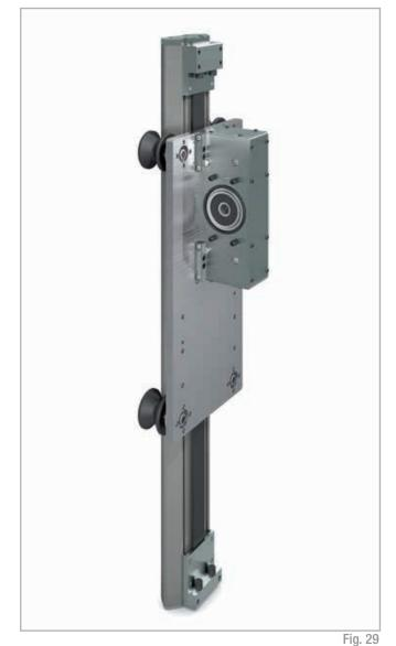
ZSY products are self-supporting extruded aluminum actuators driven by a polyurethane belt system. Due to their deep hard anodized surface treatment and their plastic compound coated rollers, ZSY series can achieve exceptionally high performances and load capacity with no maintenance or lubrication required. They also provide total reliability even in dirty environments, with uniquely quiet operation.
