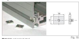
Material: galvanised steel. To be inserted through the slot. Suitable for series: MC 65
