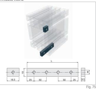
Also suitable for base-50 profiles, except A32-91 insert. Material: galvanised steel.
