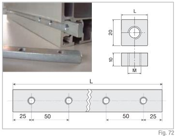
M12 (CH19) hexagonal-head screws can be used as stud bolts in profiles with 12.5 mm slots.
