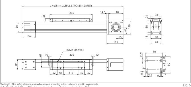
L The length of the safety stroke is provided on request according to the customer's specific requirements. \*\* For ELM80 with AC19 see PLS-11 for head length. Constant for total length calculation 554mm.
