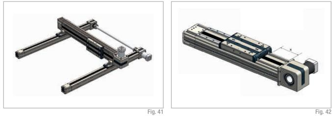
For the direct assembly of Robot linear units on other types of actuators Rollon offers dedicated assembly kits (brackets) in order to fix those brackets the ends of the actuator must be free of rails. The table below gives the codes of the assembly kit. The allowed combination of assembly as well as the length without rails at each end.
