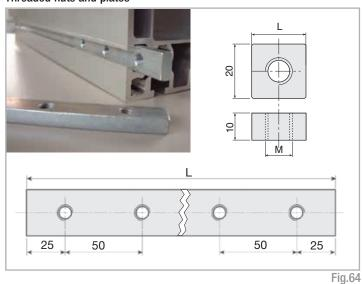
Material: galvanised steel. Suitable for series: ZC 170-220
