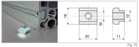
Material: galvanised steel. Suitable for series: TVS 170 - TVS 220
