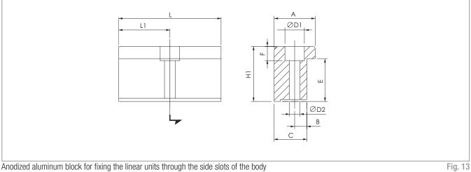
Anodized aluminum block for fixing the linear units through the side slots of the body
