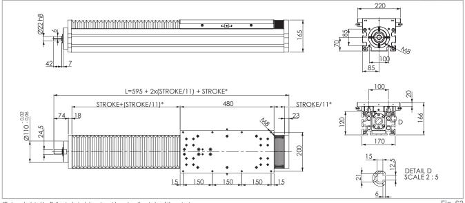
\*To be calculated by Rollon technical department based on the stroke of the actuator.
