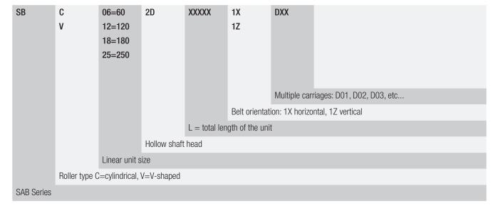
In order to create identification codes for Actuator Line, you can visit: http://configureactuator.rollon.com
