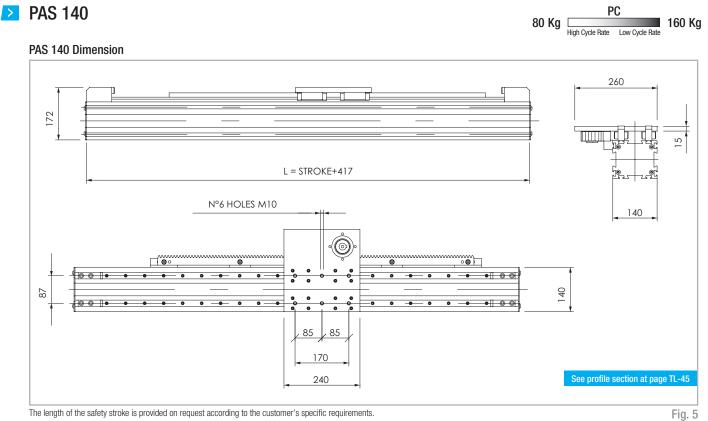
The length of the safety stroke is provided on request according to the customer's specific requirements.
