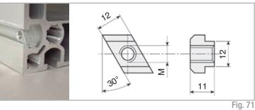
Material: galvanised steel. Suitable for series: TVS 170 - TVS 220
