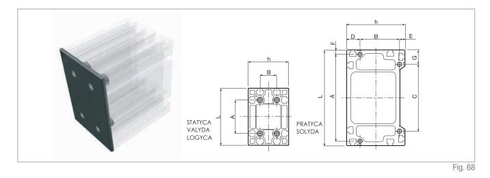
The end caps for STATYCA, VALYDA, and LOGYCA (supplied with 4 bushings 207.1892 thr. M20/6) are fixed to the profiles using the 4 holes provided in the centre that must be M20 threaded. PRATYCA and SOLYDA profiles must instead be M6 drilled and threaded as in the areas
