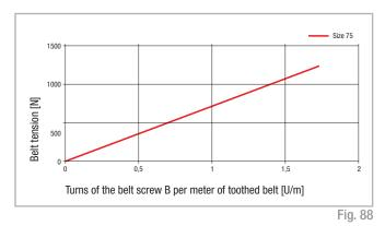
4. This means that the required number of turns is: 0.5 rpm x 2.77 m = 1.4 turns.
