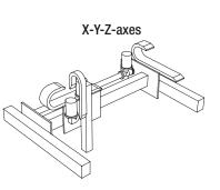
NB: The choice of X axis is based upon the actual load, the supporting points, max. deflection and the total weight of the Y-Z axes.
