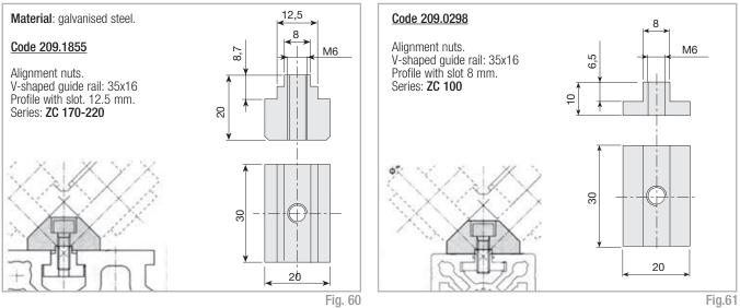
Alignment nut for slot 12.5 mm
