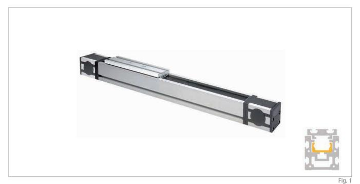
Uniline is a family of ready-to-install linear actuators. They consist of internal Compact Rail roller sliders and steel-reinforced polyurethane belts in a rigid aluminum profile. Longitudinal seals enclose the system. This arrangement provides the best protection for the actuator from soiling and damage. In the A series, the fixed bearing rail (T-rail) is mounted horizontally in the aluminum profile. Versions with long (L) or double (D) sliders in one axis are possible.
