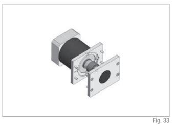
Assembly kit includes: shrink disk; adapter plate; fixing hardware
