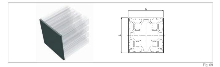
The end caps for small and medium profiles have no screws or bushes and are fitted simply by exerting moderate pressure on the end of the profile.
