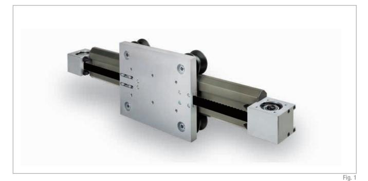
**SAB** products are self-supporting extruded aluminum actuators driven by a polyurethane belt system. Due to their deep hard anodized surface treatment and their plastic compound coated rollers, SAB series can achieve exceptionally high performances and load capacity with no maintenance or lubrication required. They also provide total reliability even in dirty environments, with uniquely quiet operation.
