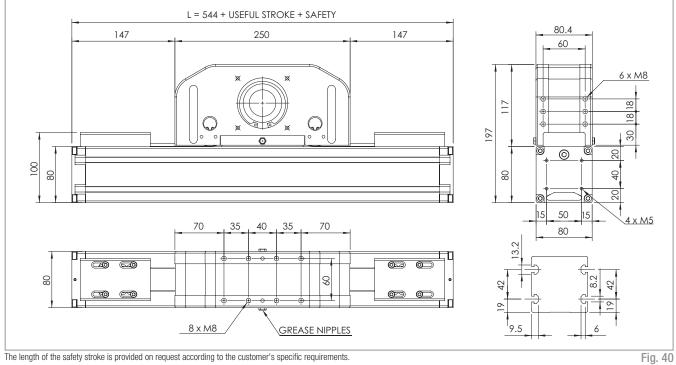
The length of the safety stroke is provided on request according to the customer's specific requirements.
