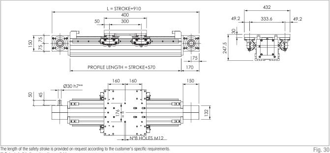
The length of the safety stroke is provided on request according to the customer's specific requirements. \*\* Output shaft is the only option available
