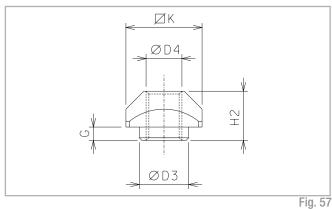
Steel nuts to be used in the slots of the body
