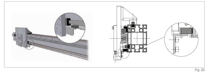
The magnetic scale is applied to the body of the module using a supporting and protective profile.
