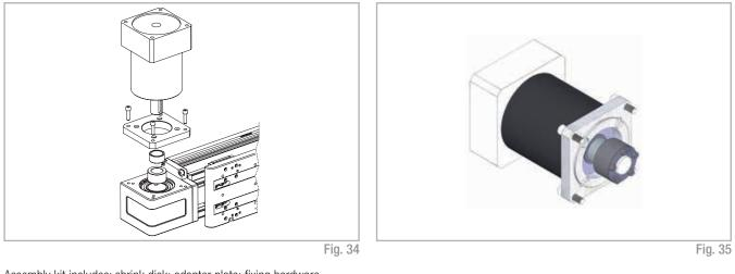
Assembly kit includes: shrink disk; adapter plate; fixing hardware
