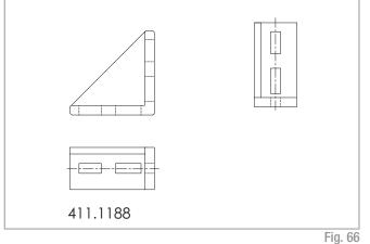
Joining bracket - Bracket 75x75x38 - Aluminum
