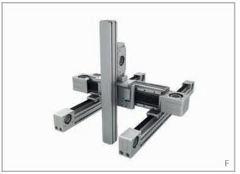
F - Linear units: X Axis 2 E-SMART - Y Axis 1 R-SMART - Z Axis 1 S-SMART Connection kit: 2 fixing brackets Kit for 2 R-SMART (Y axis) on 2 E-SMART (X axis). Connection plate Kit for S-SMART (Z axis) on 2 R-SMART (Y axis). Parallel Kit
