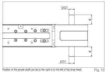
This head configuration is obtained by utilizing an assembly kit delivered as a separate accessory item.
