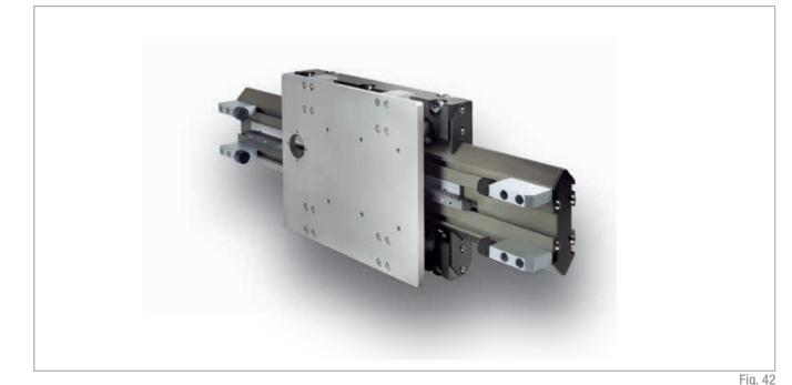
**SAR** products are self-supporting extruded aluminum actuators driven by a rack and pinion system. Due to their deep hard anodized surface treatment and their plastic compound coated rollers, SAR series can achieve exceptionally high performances and load capacity with no maintenance or lubrication required. They also provide total reliability even in dirty environments, with uniquely quiet operation.
