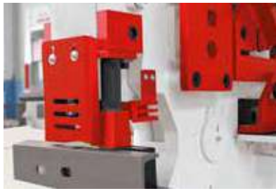
Notching station with safeguard
