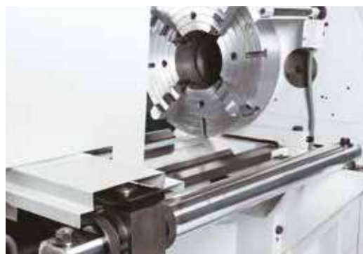
Taper turning unit is included
