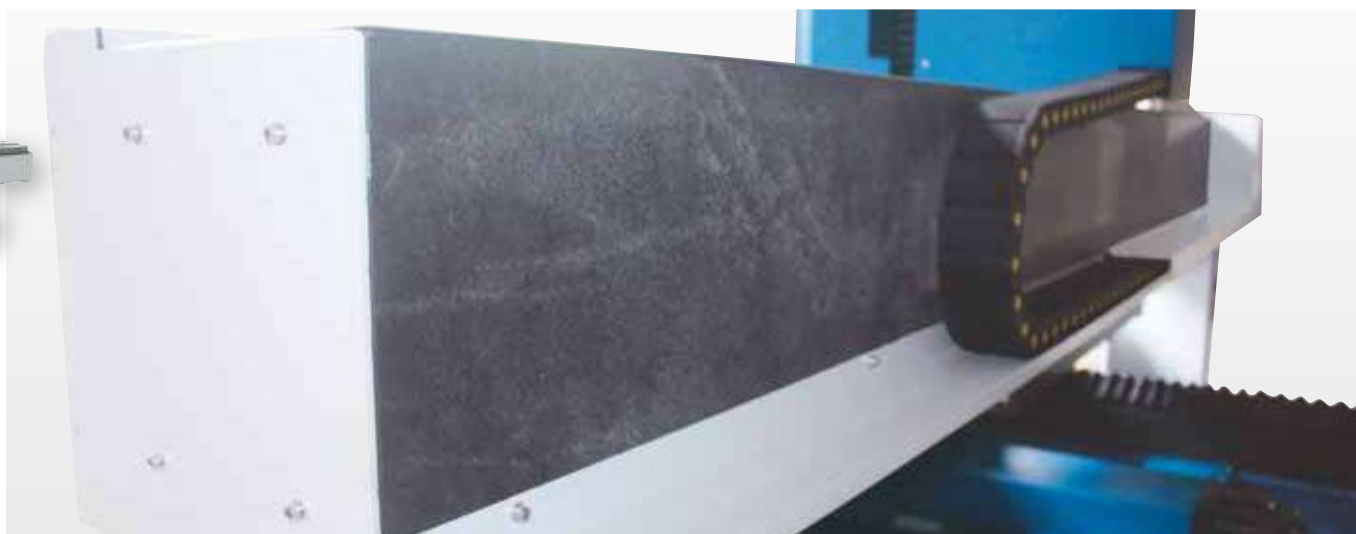
Precision-ground granite elements on all axes
