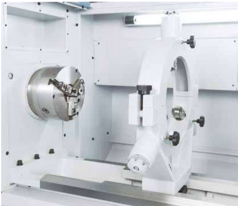
Option: steady rests up to 400 mm diameter
