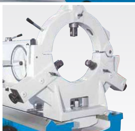
Steady rest with large capacity
