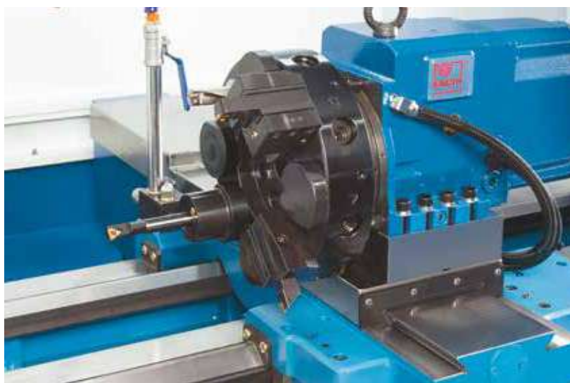
VDI 30 tool turret with 8 stations
