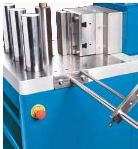
Manual side stop for batch production
