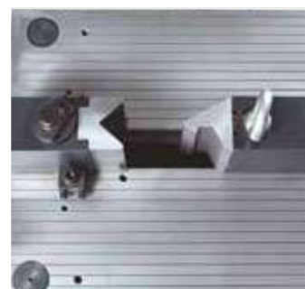
Long, supporting, hardened bending die guideways with central lubrication system
