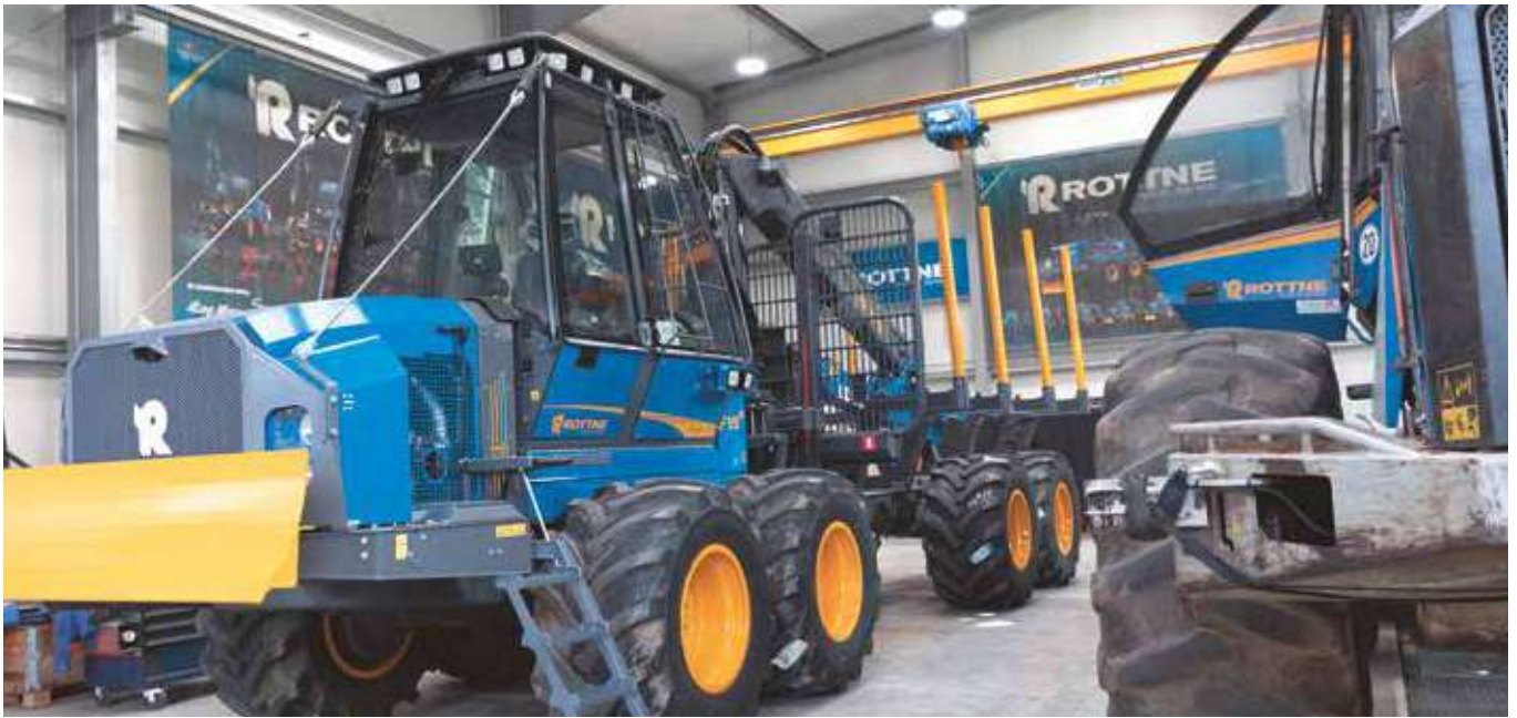
Custom crane substructure for a Rottne F15D forestry machine – a power package for high loads and long forwarders
