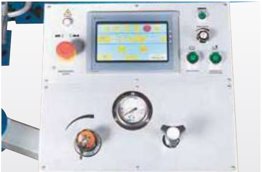
Control panel with graphic touchscreen display
