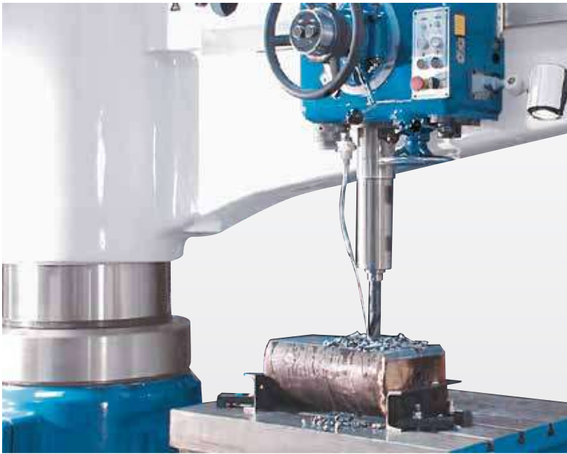
Powerful machining with automatic feed
