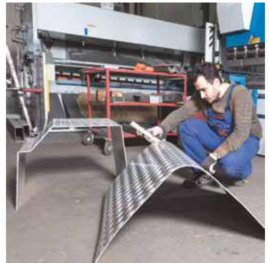
Machined component with radius for a guard cover on a timber transporter fuel tank
