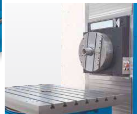
Setup table with manual rotation and manual face slide as standard
