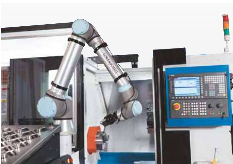
6-axis robot arm with a working radius of 1300 mm
