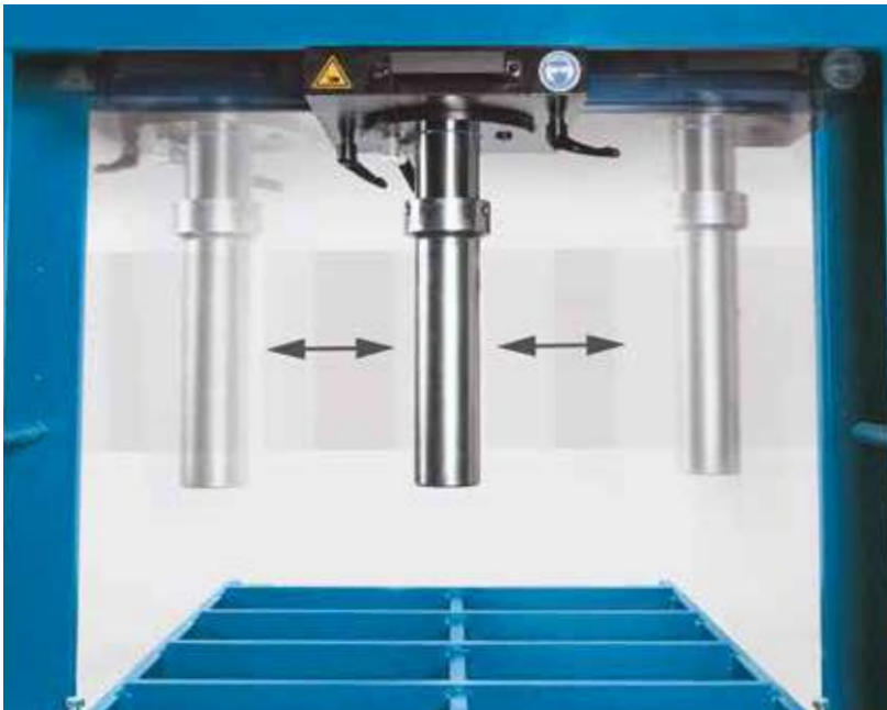
Piston unit can be moved laterally
