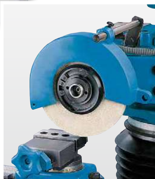
Surface grinding with angle-adjustable vise
