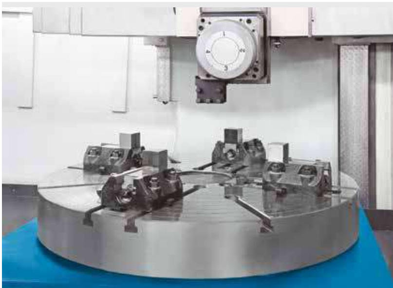
Face plate with 4-station tool changer
