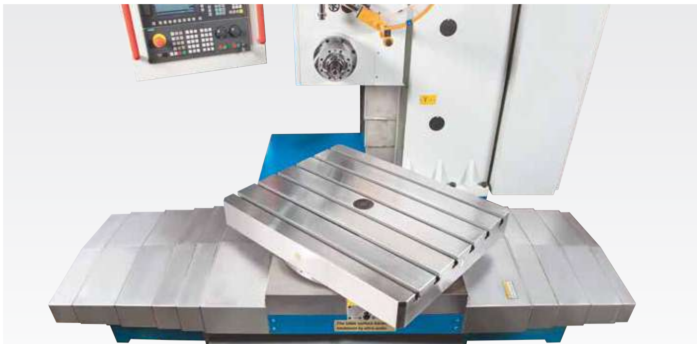
Work Table with hardened surface and 360° rotation
