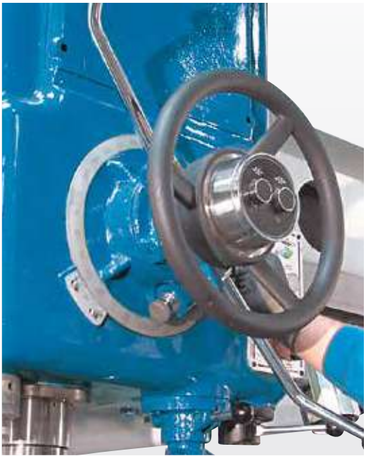
Depth stop with vernier scale
