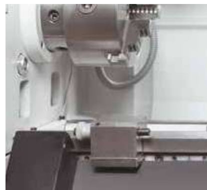
Micrometer bed stop ensures repeatability
