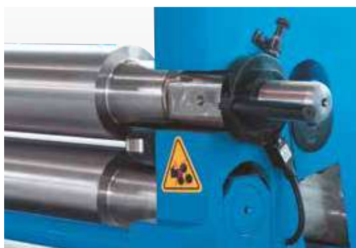
Upper roller can be swiveled out
