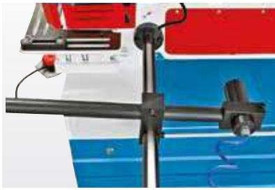
Back gauge with automatic cut activation
