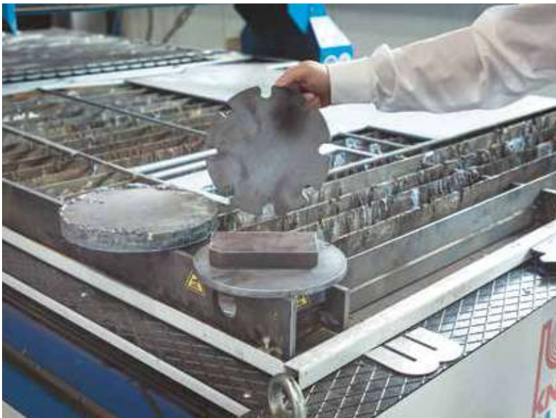
A leap forward in respect to quality: The left component has been cut with a manual plasma cutter prior to this purchase. The center part with precision cut edges was cut with the KNUTH Plasma-Jet.
