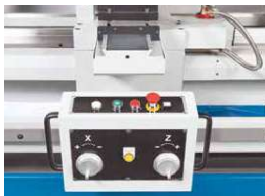
Compact control unit with electronic hand-wheels
