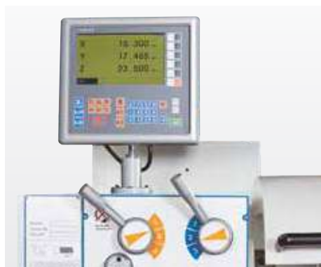
Positioning indicator on X, Z and Z1 axis
