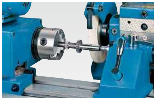
Outside cylindrical grinding for lengths up to 400 mm
