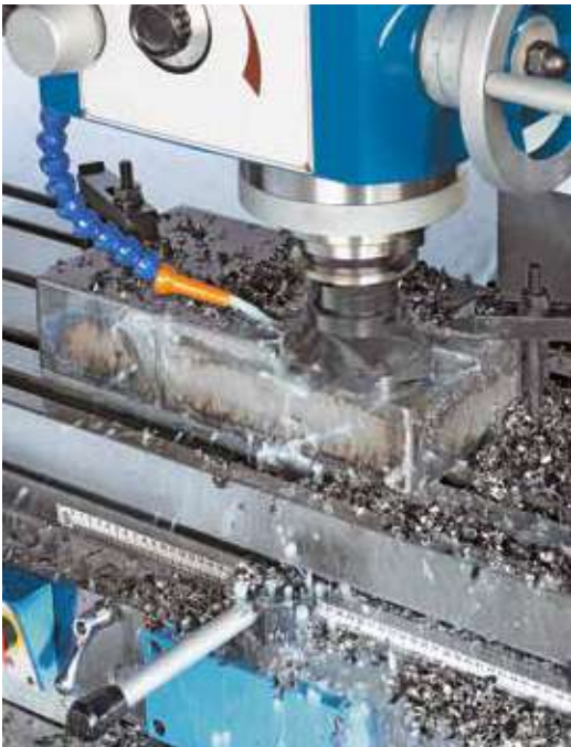
Face milling with cutter head
