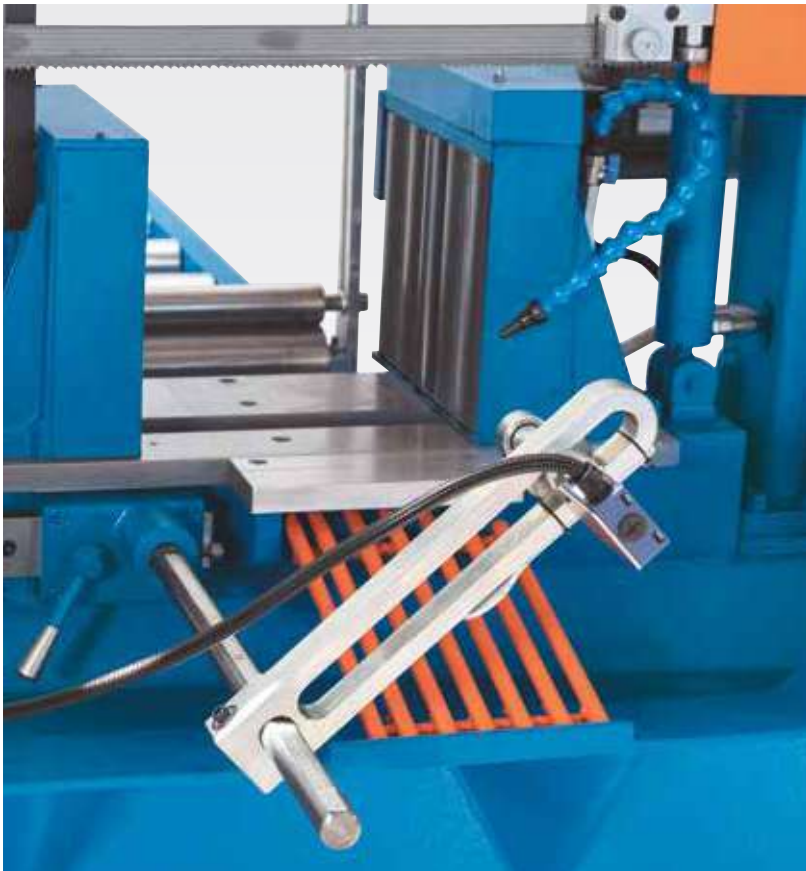
Driven feedrate rolls stop automatically when the material
