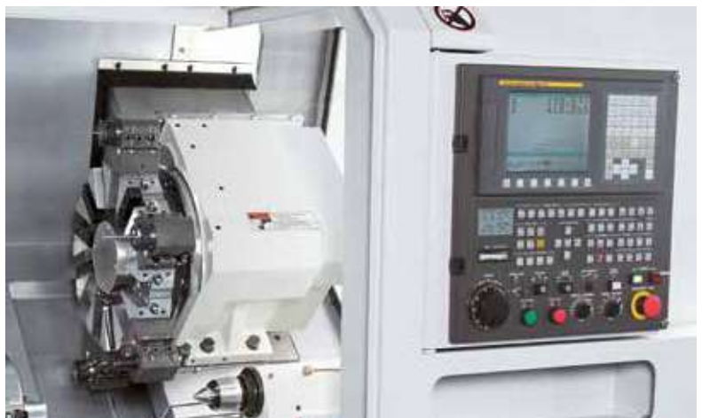
Turret with servo motor and bi-directional tool selection
