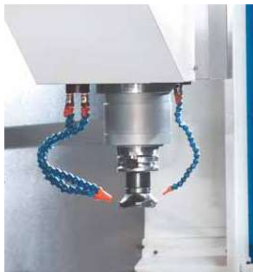
Spindle mount with cutter head
