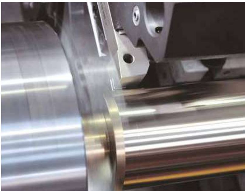
Heavy ribbing of the 45° inclined bed ensures excellent vibration damping for superior surface quality
