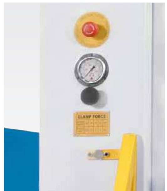
Adjustable upper die clamping pressure
