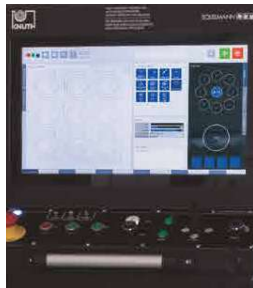
Eckelmann CNC unit with 19" touchscreen for TrueCut K models
