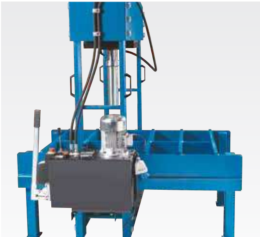
Gantry can be moved across the entire table surface
