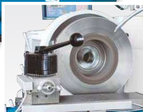
Turnado V: Constant cutting speed for flawless surfaces
