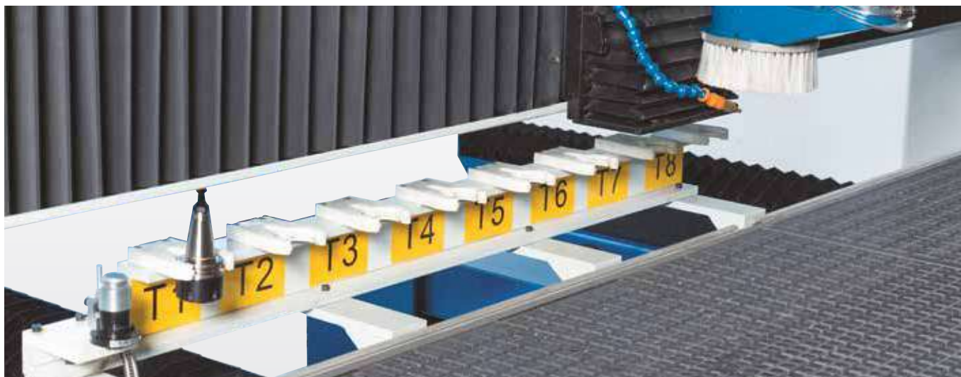
Linear 8-station tool changer
