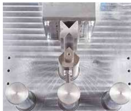
Angle lines are engraved in the work table for easy orientation
