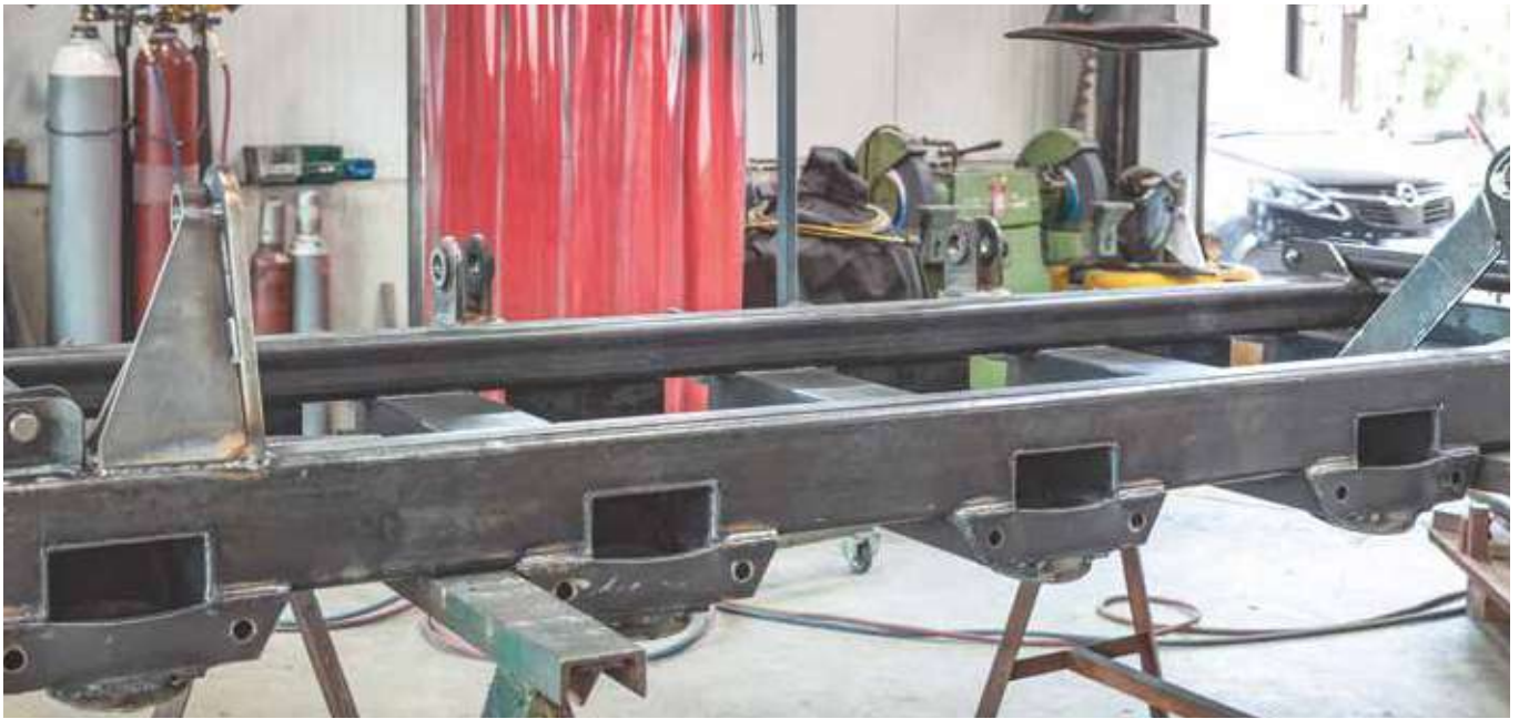
One finished part welded from a variety of cut parts that were produced with a KNUTH Plasma-Jet
