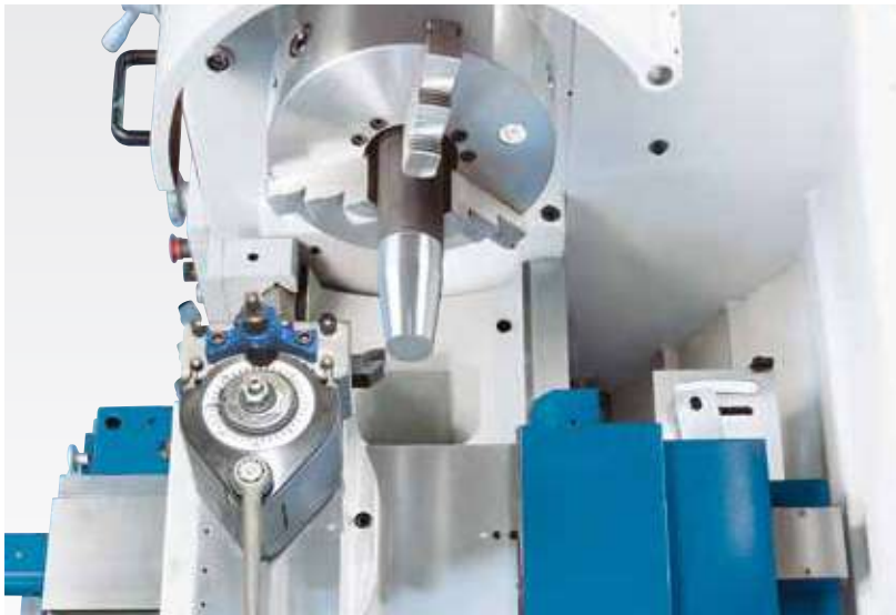
Taper turning unit is included
