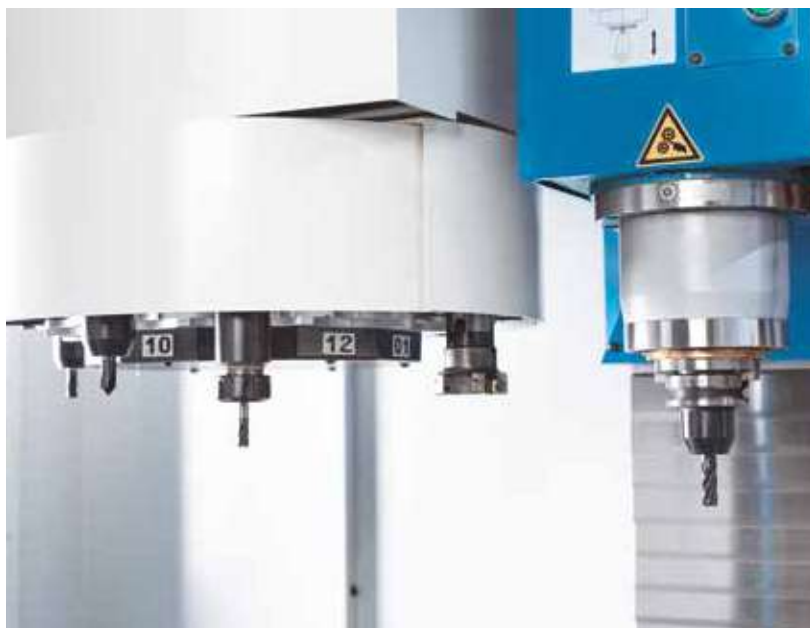
Rugged horizontal tool changer with 12 stations
