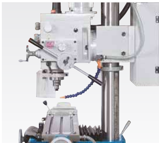
Automatic quill feed with 3-step gears
