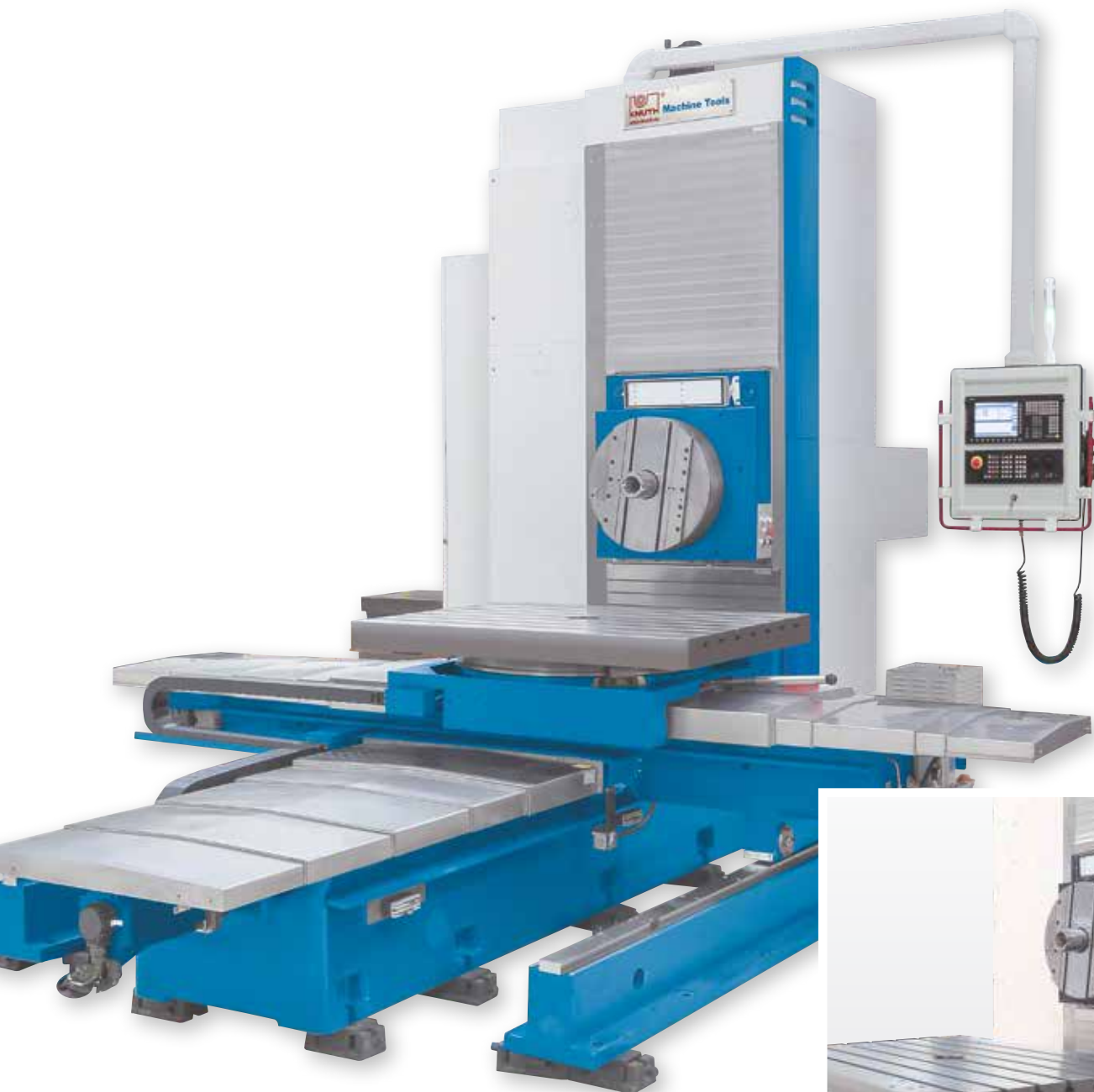
Setup table with manual rotation and manual face slide as standard
