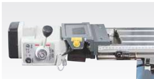
Infinitely variable milling table feed
