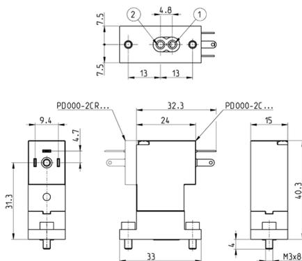
For vacuum applications connect the suction source to port 2
