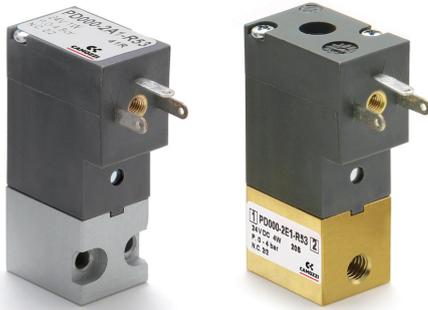
The Series PD directly operated solenoid valves are available in the 2/2-way normally closed (NC) version. Pneumatic interfaces allow installation on manifolds in horizontal or vertical position. Also available with threaded connections.
