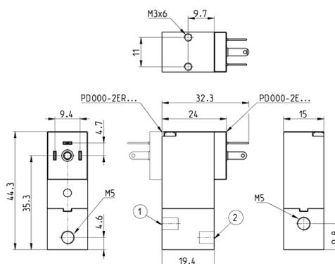
For vacuum applications connect the suction source to port 2
