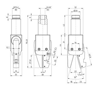
A = connection port B = fixing thread C = sensor fixing hole
