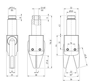
A = connection port B = fixing thread
