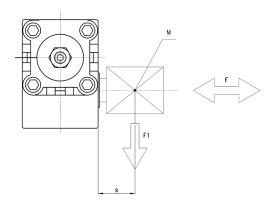
M = Center of gravity of the applied theoretical load F = Axial load (N)
