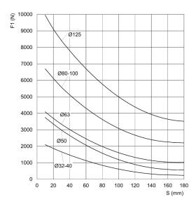
Max. radial load F1 with F = 0 S = distance between actuator and center of gravity of the applied theoretical load (mm)
