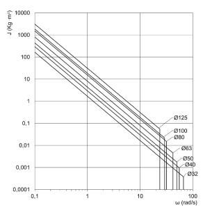
Maximum energy that can be cushioned according to the angular speed. J = Moment of inertia (Kg · m<sup>2</sup>)  $\omega$  = Angular speed (rad/s)
