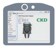
The digital I/O can be configured while viewing a graphic display of the gripper's open/closed status.
