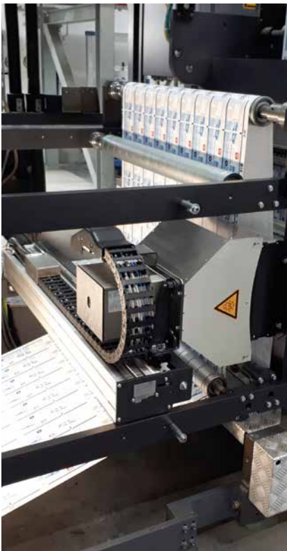
ELSCAN OMS6 on flexo printing machine
