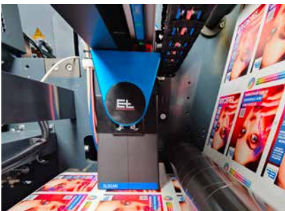
ELSCAN OMS5 on digital printing machine
