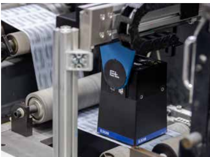
ELSCAN OMS5 on label printing machine
