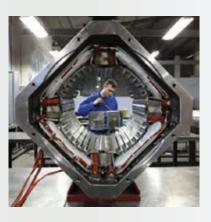
In standard version, all motors have separate excitation, the field being shunt wound. Compound or series winding can be supplied on request.
