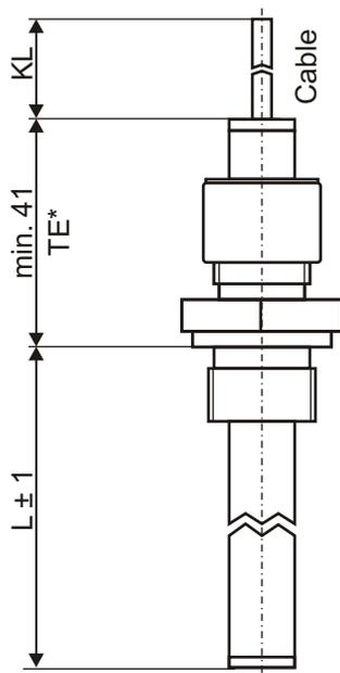
(TE) Depth setting on the screw connection can be selected by the customer
