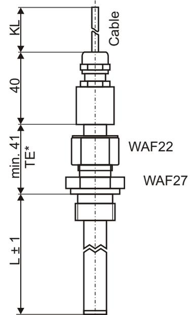
(TE) Depth setting on the screw connection can be selected by the customer
