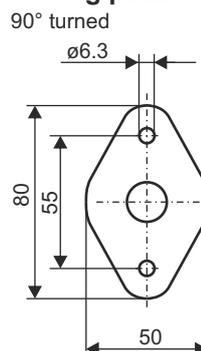
Connection: right-angled socket 3-pole + PE
