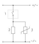
There is no protection on the Reed sensors on the inductive load, therefore it is advisable to use electric circuits with protection against the voltage spikes: the first for direct current (DC), the second for alternating current (AC).
