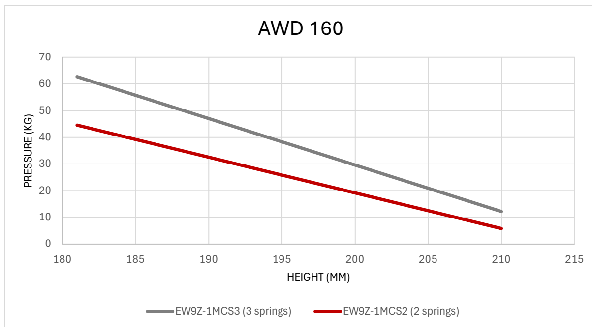
Figure 13 - Height tolerance and pressure level for AWD® 160
