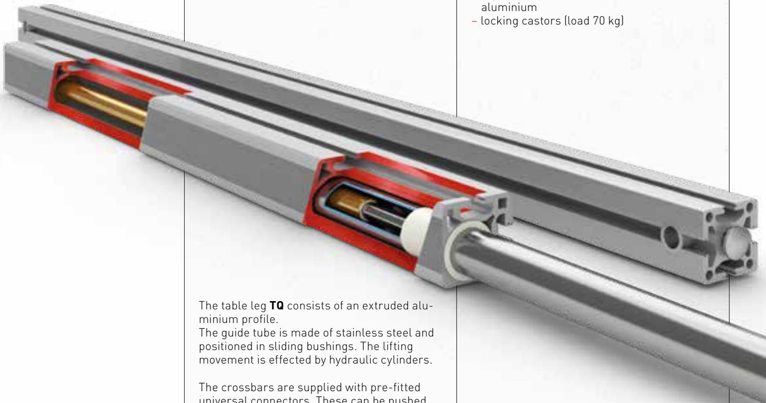
The table leg **TQ** consists of an extruded aluminium profile. The guide tube is made of stainless steel and positioned in sliding bushings. The lifting movement is effected by hydraulic cylinders.
