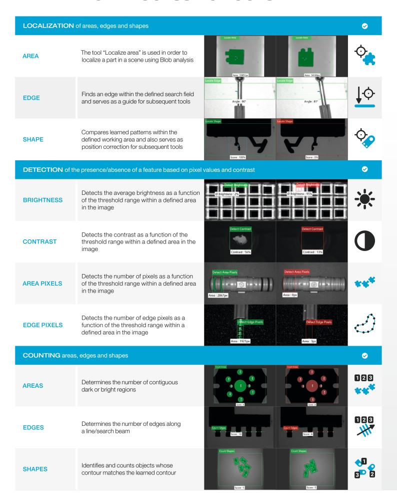
Via comprehensive image processing tools, both the verification of the quality and completeness of parts is possible as well as their localization and the transmission of determined positions by way of various communication interfaces. Demanding tasks, such as quality inspections of highly reflective objects and applications in changing ambient lighting situations or at high speeds are reliably performed.
