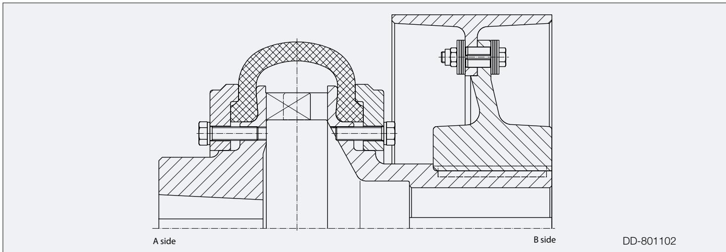
Shaft couplings in accordance with the standards of the metallurgical plants for double-cheek brakes according to DIN 15435.
