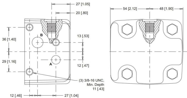
**B** Main Ports **A:** 12.7 [.500] Drilled **B:** 15.9 [.625] Drilled
