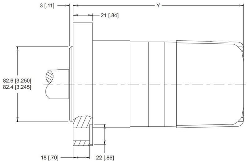
Figure 14 4-Hole, Magneto Mount
