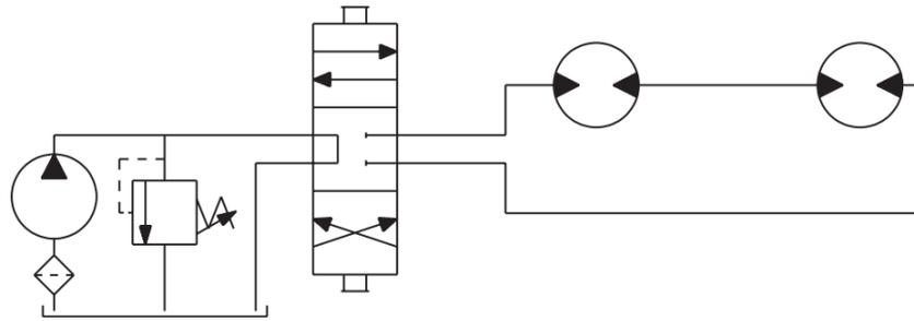
Figure 2 Series Circuit
