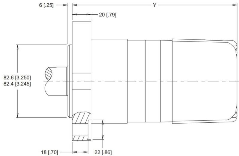
Figure 15 4-Hole, SAE A Mount
