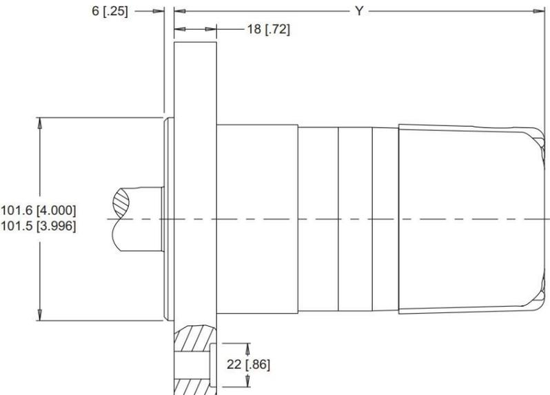
Figure 16 2-Hole, SAE B Mount
