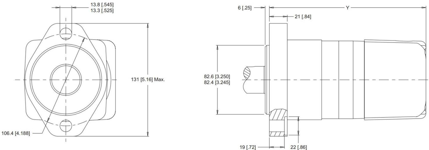
Figure 13 2-Hole, SAE A Mount
