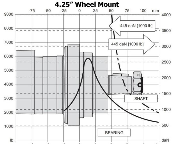
Figure 19 4.25" Wheel Mount Allowable Shaft Load/Bearing Curve
