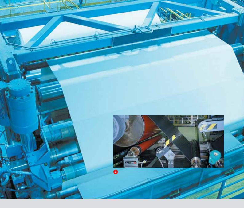
**1** Production of abrasive paper. This equipment measures tension and controls the intermediate drive.
