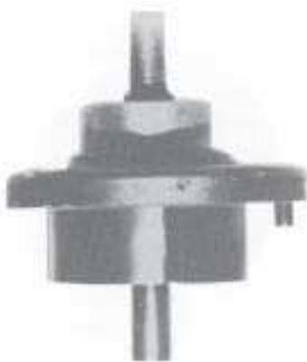
Figure 25 Clearance between an air motor's rotor and end plates of the housing are very small, as this photo shows. Misalignment could close the clearance, causing the rotor in bind and turn with difficulty or not at all.
