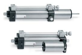
Series 43 hydrocheck units are available with two different types of control: regulated outward movement and fast return; or fast outward movement and regulated return. These hydrochecks come complete with an oil surge tank which ensures automatic equalisation. Speed variation is obtained by means of an incorporated flow regulator designed to allow comprehensive and constant use.
